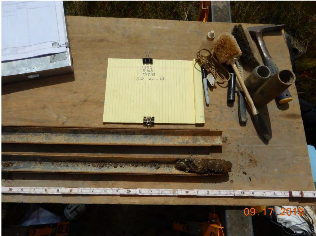
Photograph 48: B-105A(P); S-2 from 2.0 to 3.5 feet. Clayey Sand with Gravel [Alluvium/Colluvium].
