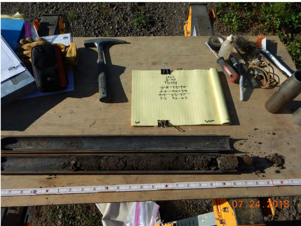
Photograph 19: B-102A(P); S-5 from 9.0 to 10.5 feet. Clayey Gravel with Sand [Fill].
