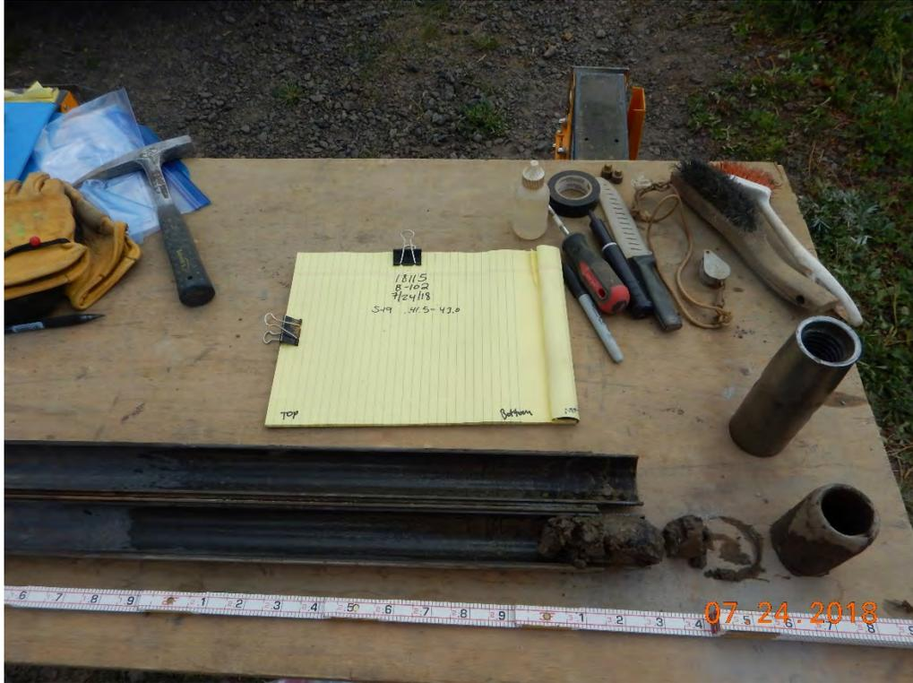
Photograph 30: B-102A(P); S-19 from 41.5 to 43.0 feet. Clayey Sand with Gravel [Fill].
