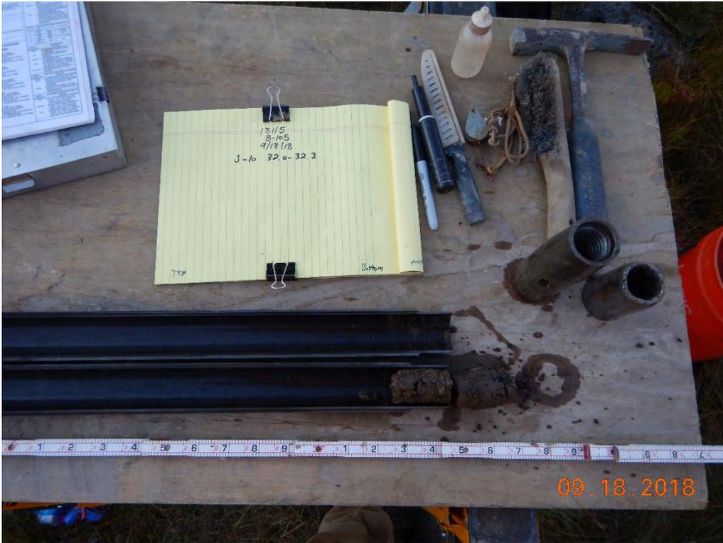
Photograph 56: B-105A(P); S-10 from 32.0 to 32.3 feet. Sandy Lean Clay [Alluvium/Colluvium].
