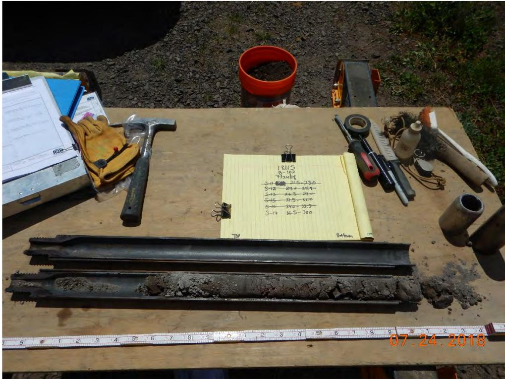
Photograph 28: B-102A(P); S-17 from 36.5 to 38.0 feet. Clayey Gravel with Sand [Fill].
