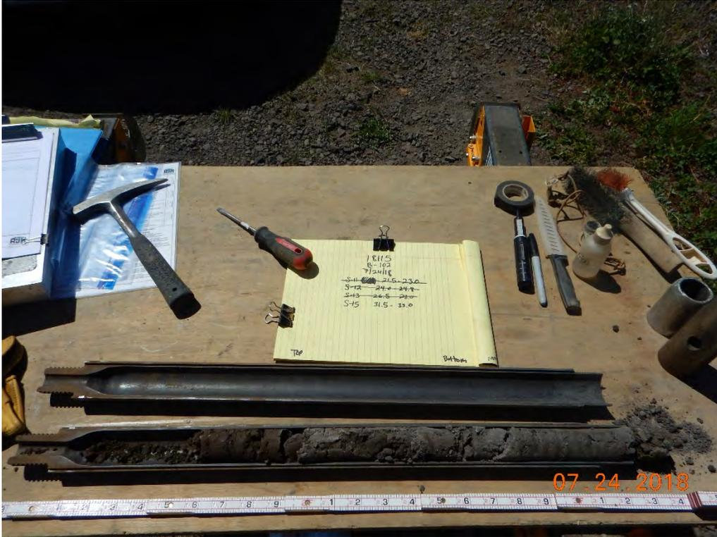
Photograph 26: B-102A(P); S-15 from 31.5 to 33.0 feet. Clayey Gravel with Sand [Fill].
