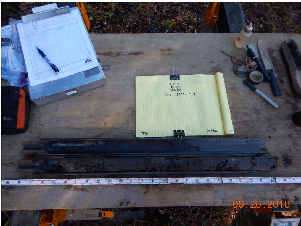
Photograph 44: B-104(P); S-5 from 13.4 to 14.9 feet. Sandy Lean Clay with Gravel [Alluvium/Colluvium].
