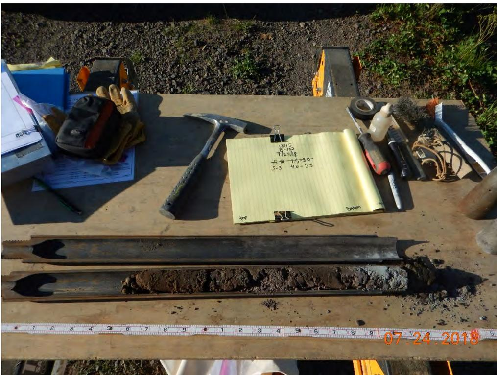
Photograph 17: B-102A(P); S-3 from 4.0 to 5.5 feet. Clayey Gravel with Sand [Fill].
