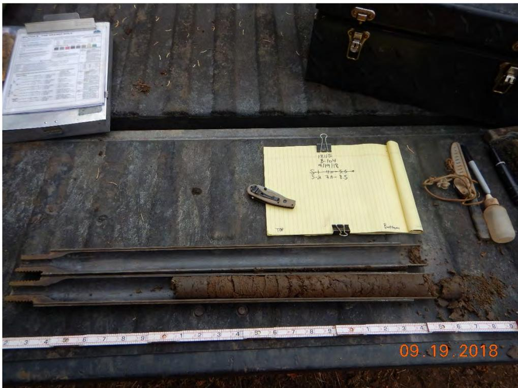
Photograph 42: B-104(P); S-2 from 4.0 to 5.5 feet. Sandy Lean Clay with Gravel [Alluvium/Colluvium].
