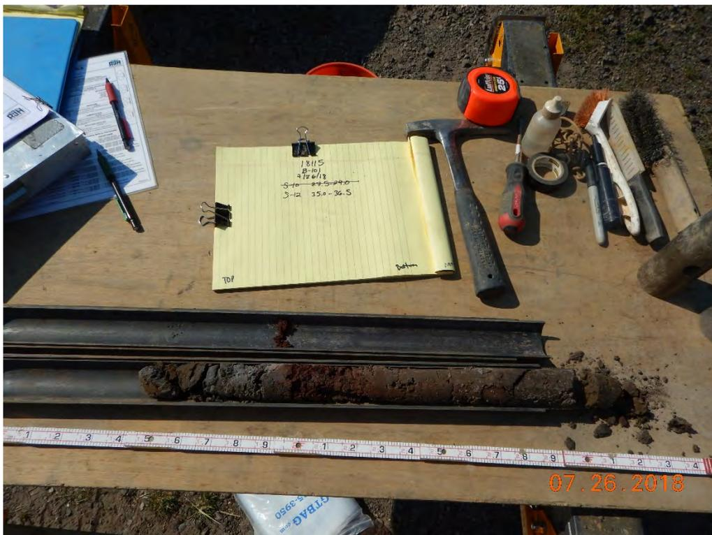
Photograph 8: B-101(P); S-12 from 35.0 to 36.5 feet. Clayey Sand with Gravel [Fill].
