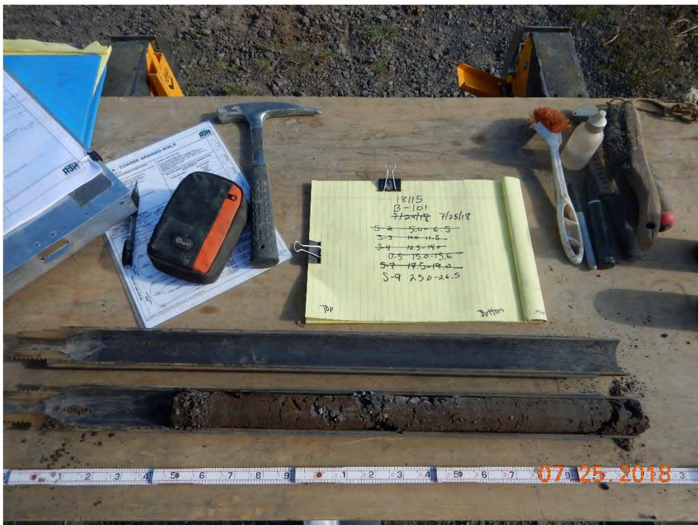
Photograph 6: B-101(P); S-9 from 25.0 to 26.5 feet. Clayey Sand with Gravel [Fill].
