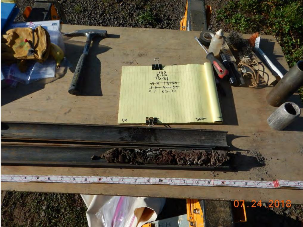
Photograph 18: B-102A(P); S-4 from 6.5 to 8.0 feet. Clayey Gravel with Sand [Fill].
