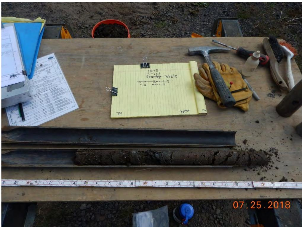
Photograph 2: B-101(P); S-3 from 10.0 to 11.5 feet. Clayey Sand with Gravel [Fill].
