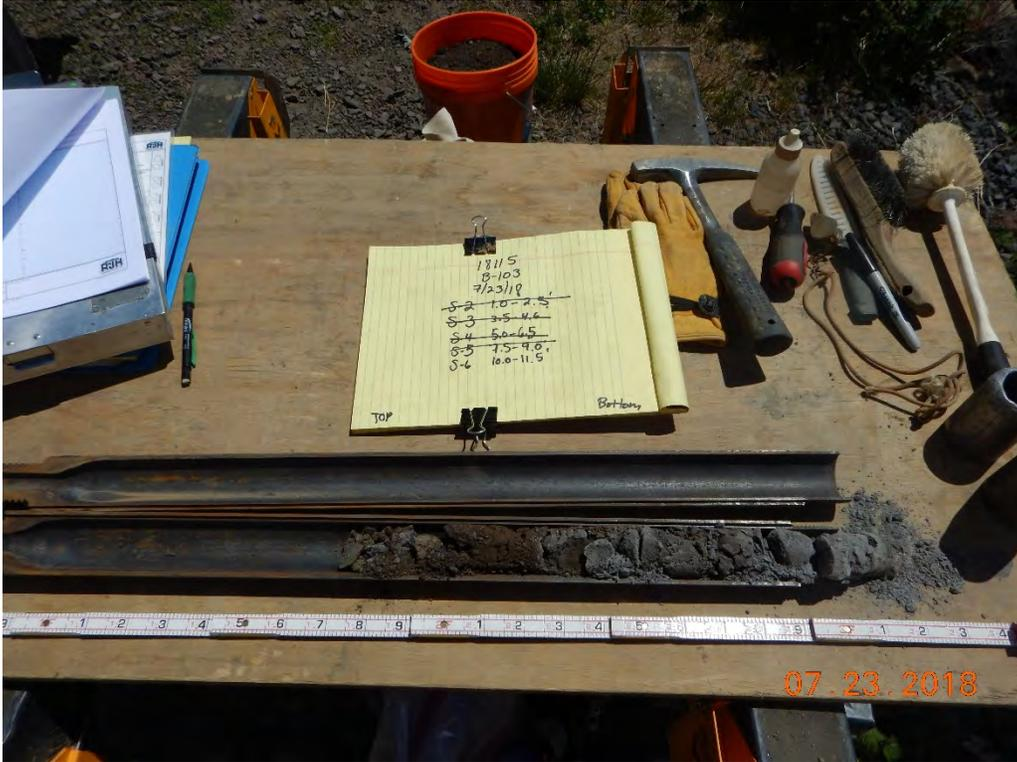
Photograph 36: B-103(P); S-6 from 10.0 to 11.5 feet. Clayey Sand with Gravel [Fill].
