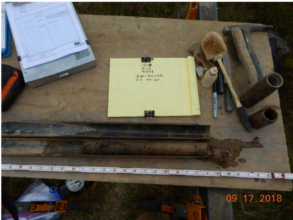
Photograph 49: B-105A(P); S-3 from 4.5 to 6.0 feet. Clayey Sand with Gravel [Alluvium/Colluvium].
