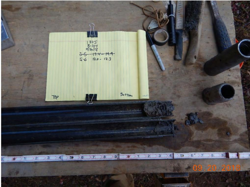
Photograph 45: B-104(P); S-6 from 17.0 to 17.3 feet. Gravelly Lean Clay with Sand [Alluvium/Colluvium].
