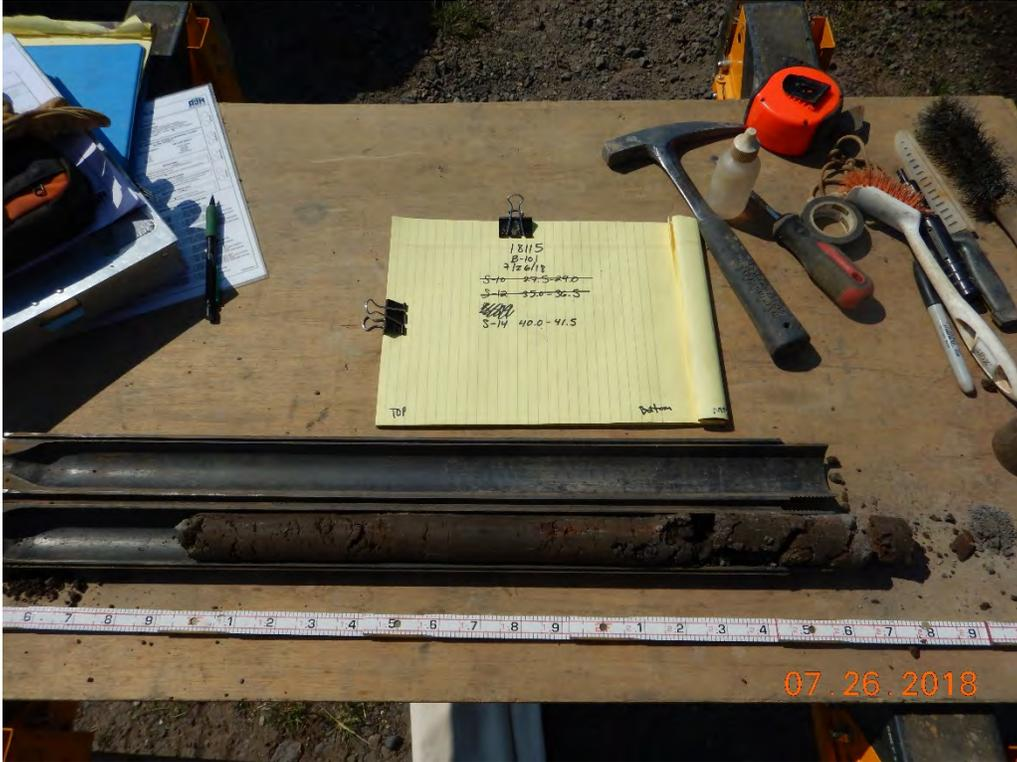
Photograph 9: B-101(P); S-14 from 40.0 to 41.5 feet. Clayey Sand with Gravel [Fill].
