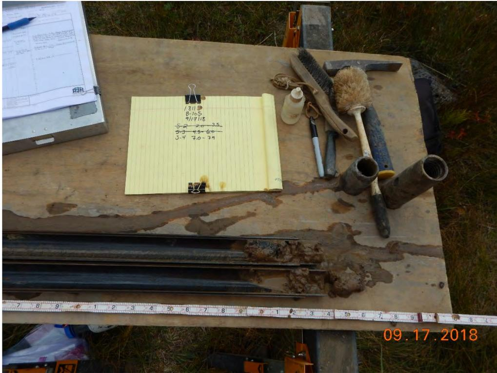
Photograph 50: B-105A(P); S-4 from 7.0 to 7.9 feet. Clayey Sand with Gravel [Alluvium/Colluvium].
