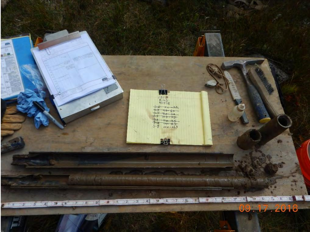
Photograph 54: B-105A(P); S-8 from 22.0 to 23.5 feet. Lean Clay [Alluvium/Colluvium].
