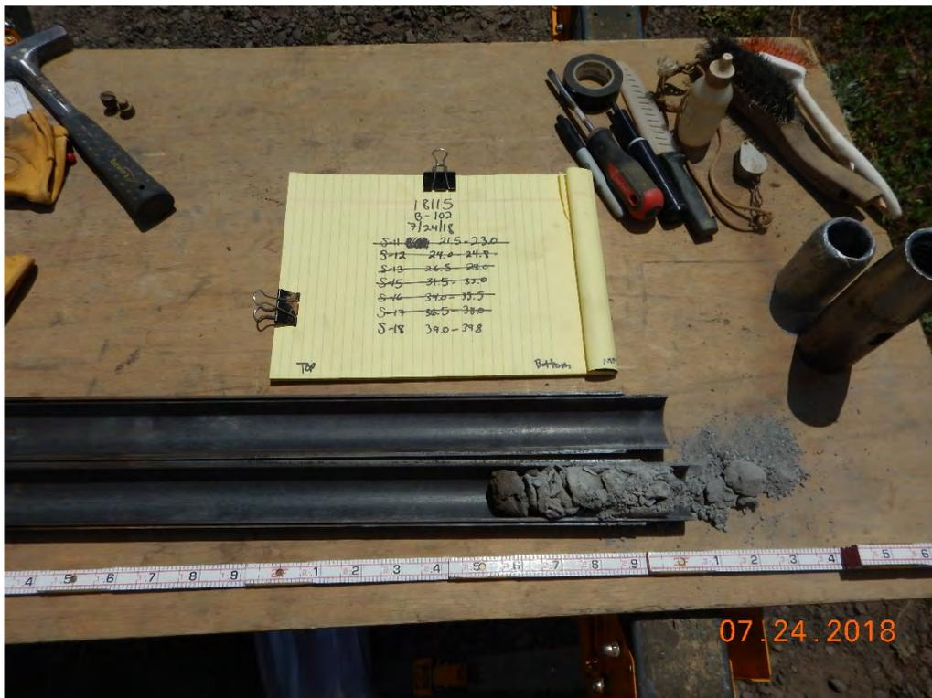
Photograph 29: B-102A(P); S-18 from 39.0 to 39.8 feet. Poorly Graded Gravel with Clay and Sand [Fill].
