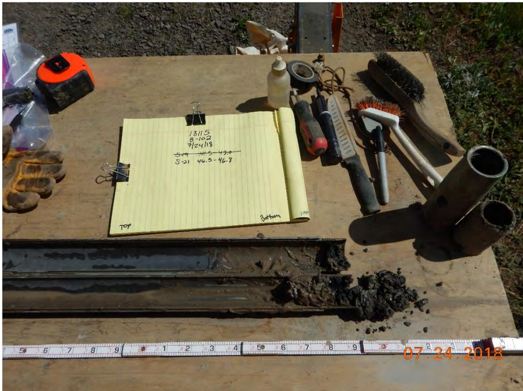
Photograph 31: B-102A(P); S-21 from 46.5 to 46.8 feet. Poorly Graded Gravel with Clay and Sand [Fill].
