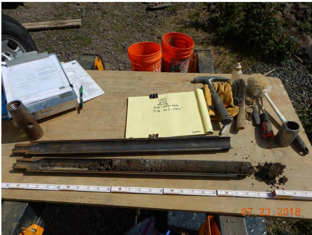
Photograph 39: B-103(P); S-12 from 22.5 to 24.0 feet. Clayey Sand with Gravel [Fill]. Gravelly Lean Clay with Sand [Alluvium/Colluvium].
