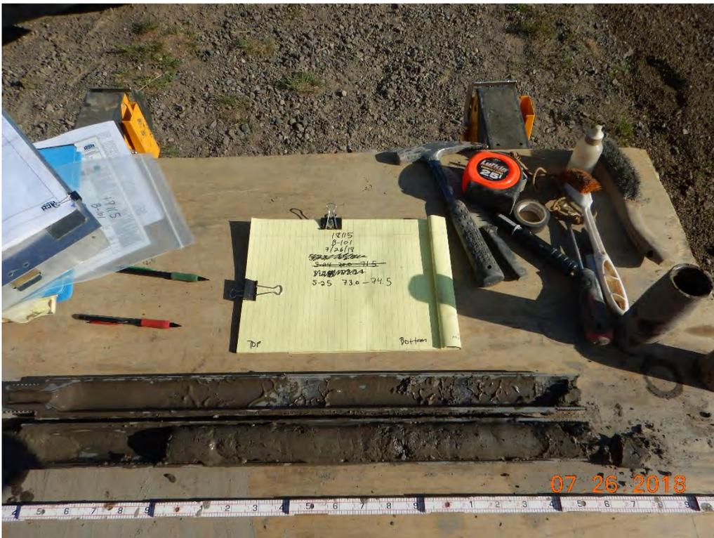
Photograph 14: B-101(P); S-25 from 73.0 to 74.5 feet. Sandy Lean Clay [Alluvium/Colluvium].
