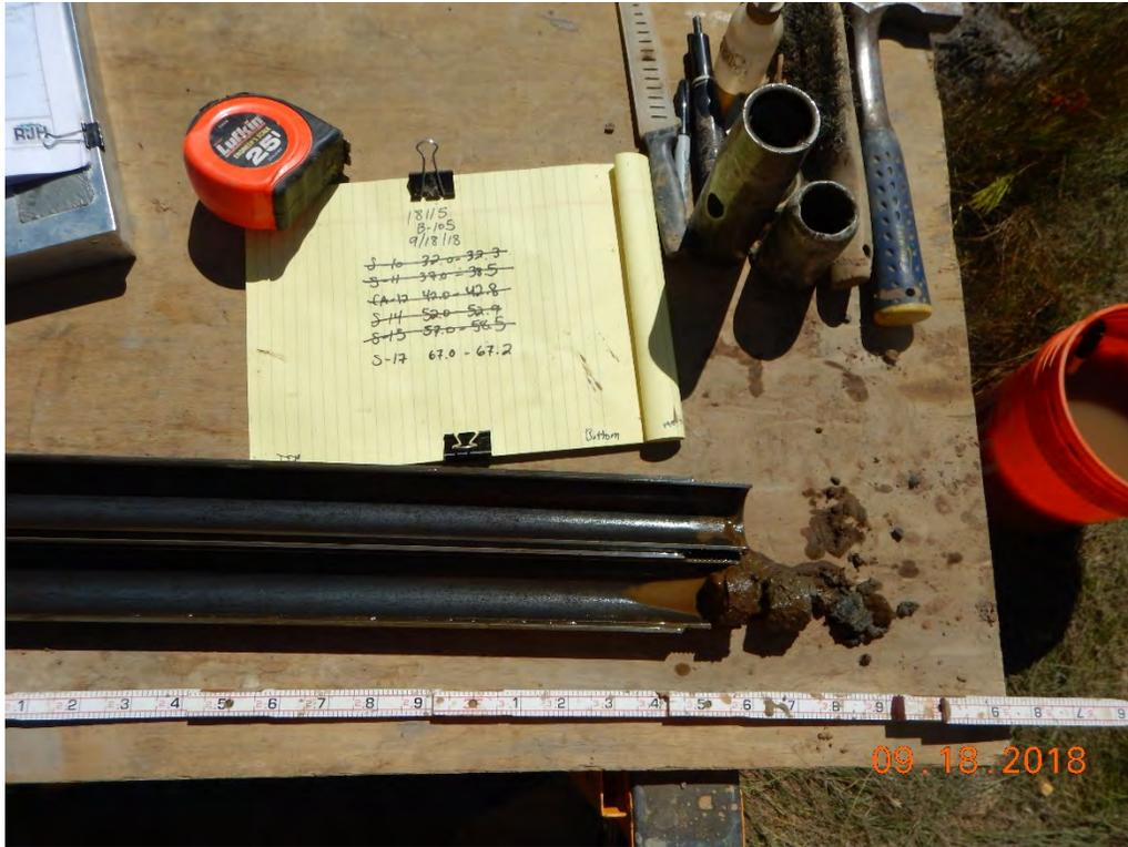
Photograph 60: B-105A(P); S-17 from 67.0 to 67.2 feet. Clayey Sand with Gravel [Alluvium/Colluvium].
