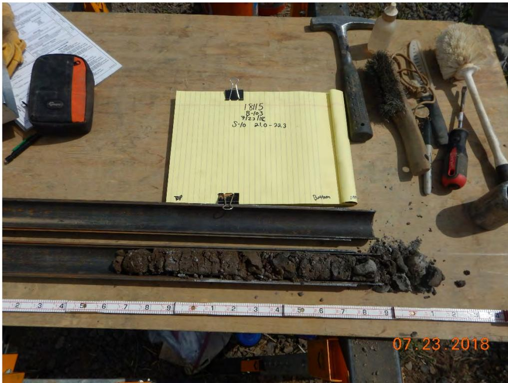
Photograph 38: B-103(P); S-10 from 21.0 to 22.3 feet. Clayey Sand with Gravel [Fill].
