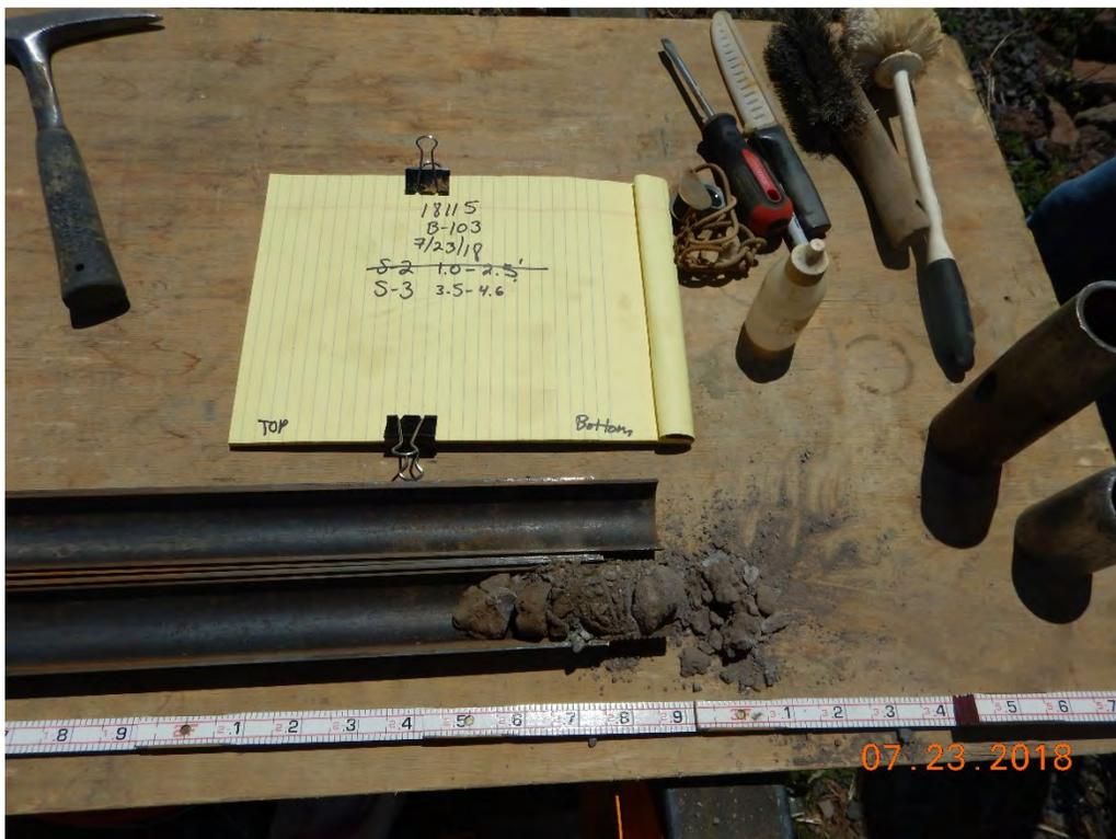
Photograph 33: B-103(P); S-3 from 3.5 to 4.6 feet. Clayey Gravel with Sand [Fill].
