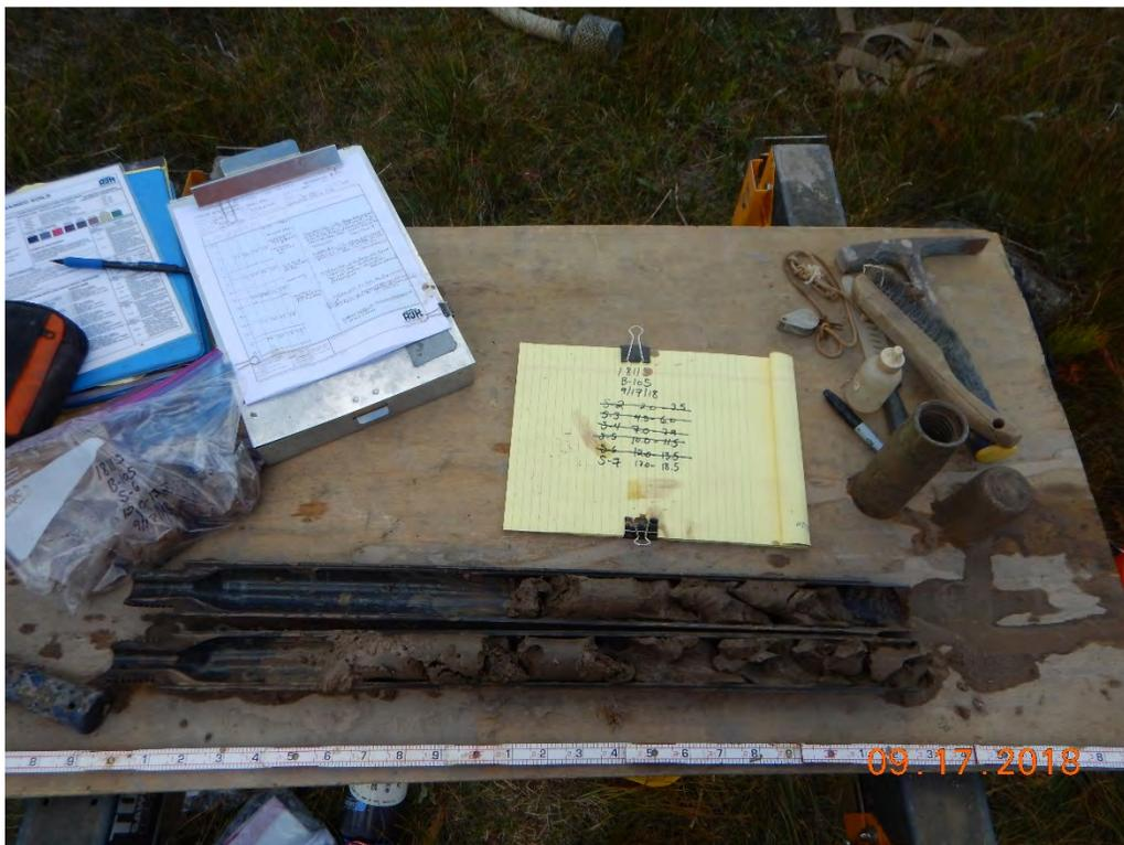
Photograph 53: B-105A(P); S-7 from 17.0 to 18.5 feet. Lean Clay with Sand [Alluvium/Colluvium].
