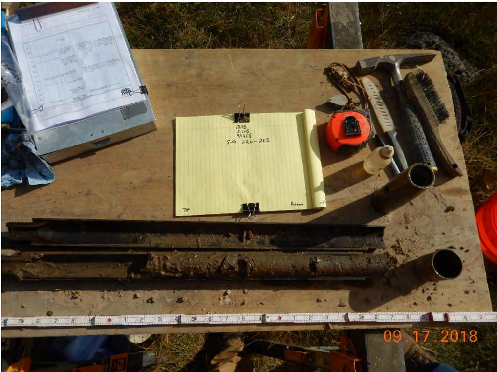
Photograph 55: B-105A(P); S-9 from 27.0 to 28.5 feet. Sandy Lean Clay with Gravel [Alluvium/Colluvium].
