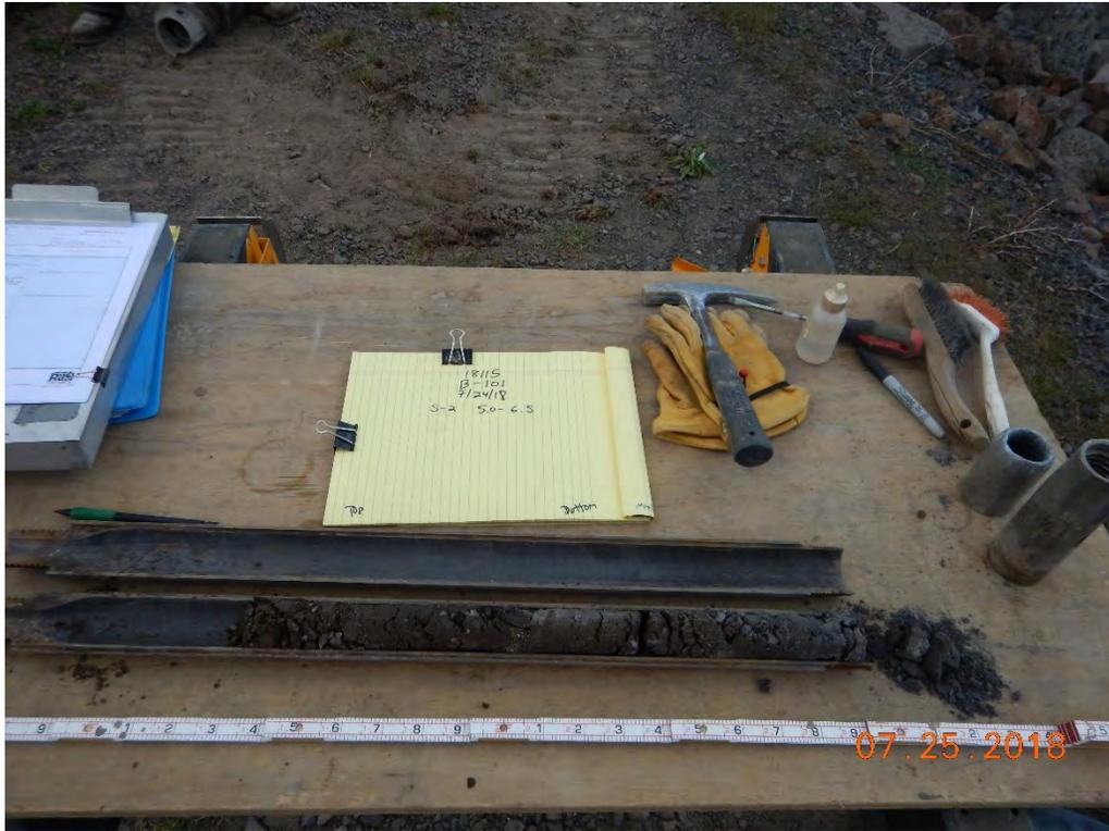
Photograph 1: B-101(P); S-2 from 5.0 to 6.5 feet. Clayey Gravel with Sand [Fill].
