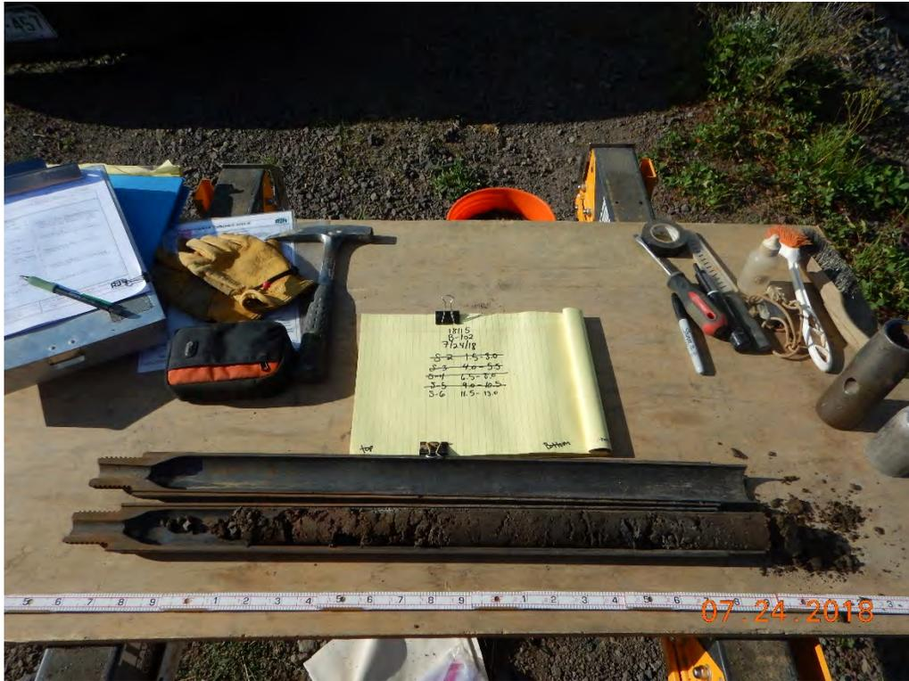
Photograph 20: B-102A(P); S-6 from 11.5 to 13.0 feet. Clayey Gravel with Sand [Fill].
