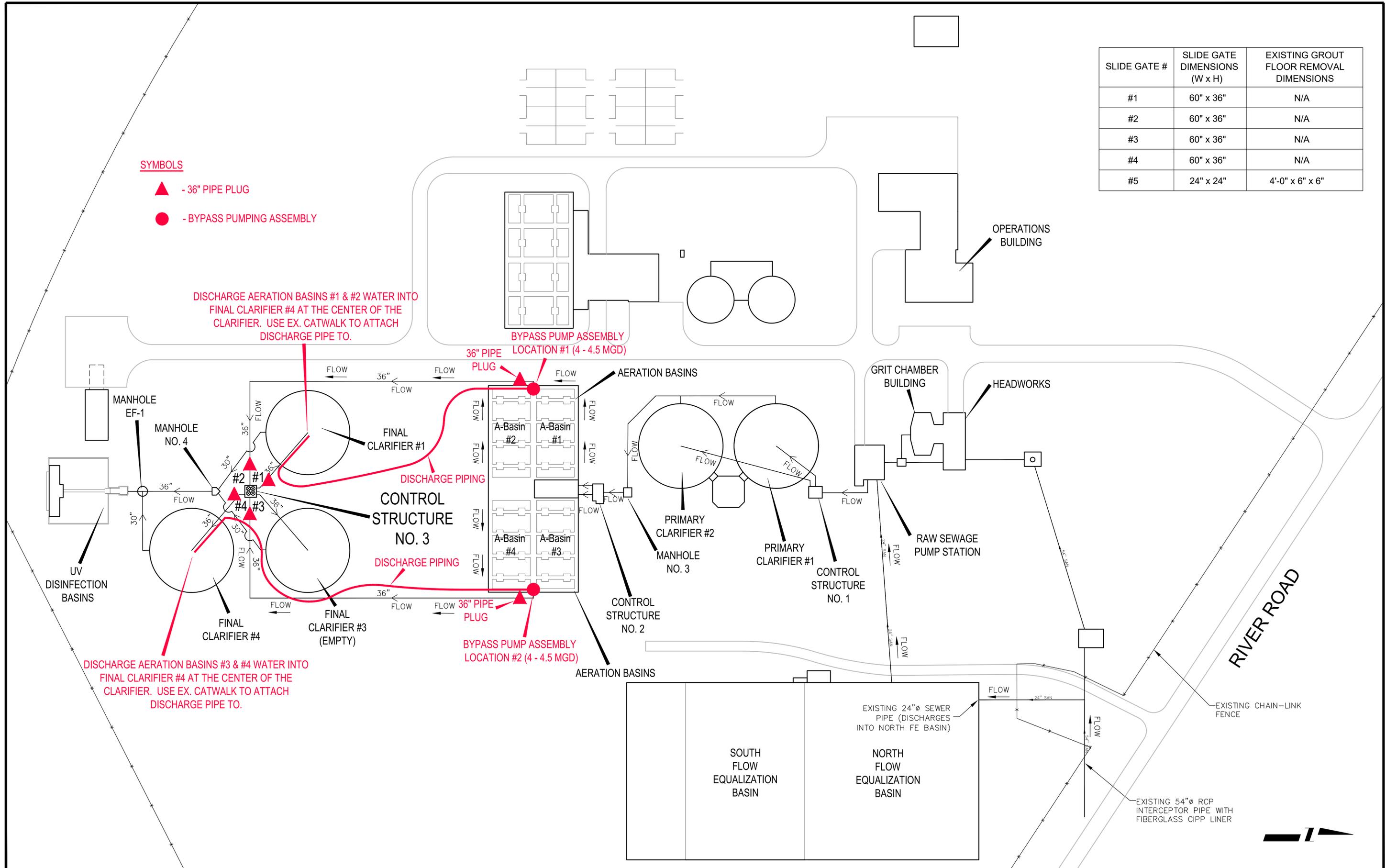
DISCHARGE AERATION BASINS #1 & #2 WATER INTO FINAL CLARIFIER #4 AT THE CENTER OF THE CLARIFIER. USE EX. CATWALK TO ATTACH DISCHARGE PIPE TO.
