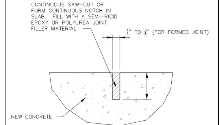
NOTE: REFER TO OTHER TYPICAL DETAILS FOR SLAB REINFORCING REQUIREMENTS. PROVIDE METZGER/McQUIRE MM-80 SEMI-RIGID EPOXY JOINT FILLER OR REZI-WELD FLEX, SEMI-RIGID EPOXY JOINT FILLER (FILLER WILL NOT BE PAID SEPARATELY BUT SHALL BE INCLUDED IN THE WORK).
