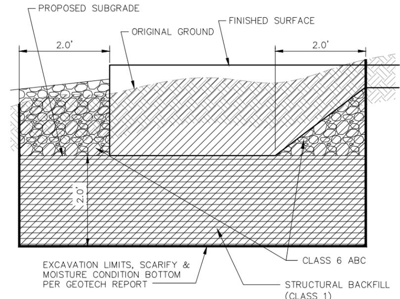
**D.1** CONCRETE EXT. WALL FTG. EXCAVATION DTL.
