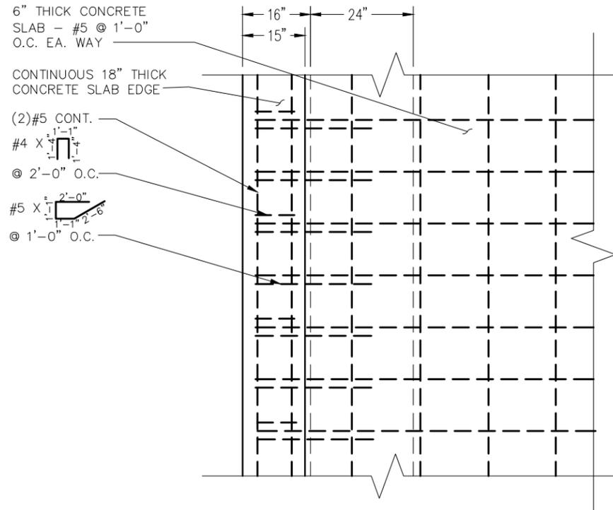
**C.1** TYPICAL SLAB DETAIL - PLAN THICKENED EDGE WITH STEM WALL
