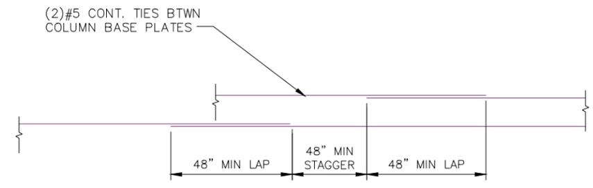
**C.3** TYPICAL TENSION TIE DETAIL - PLAN
