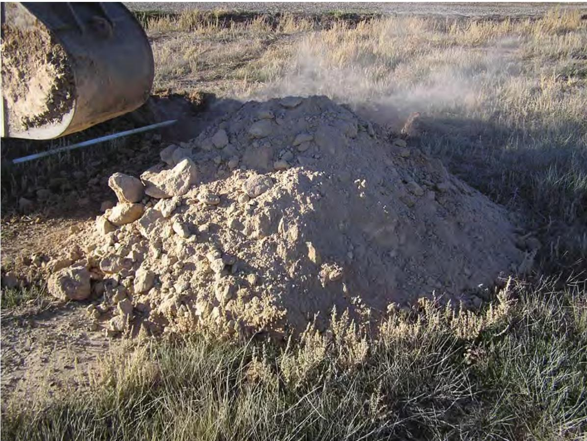
The top 1 ½ foot was generally consistent with that of a sandy clay (CL) material. 1 ½ - 4 feet the material was a very fine sand /rock flour material (ML).
