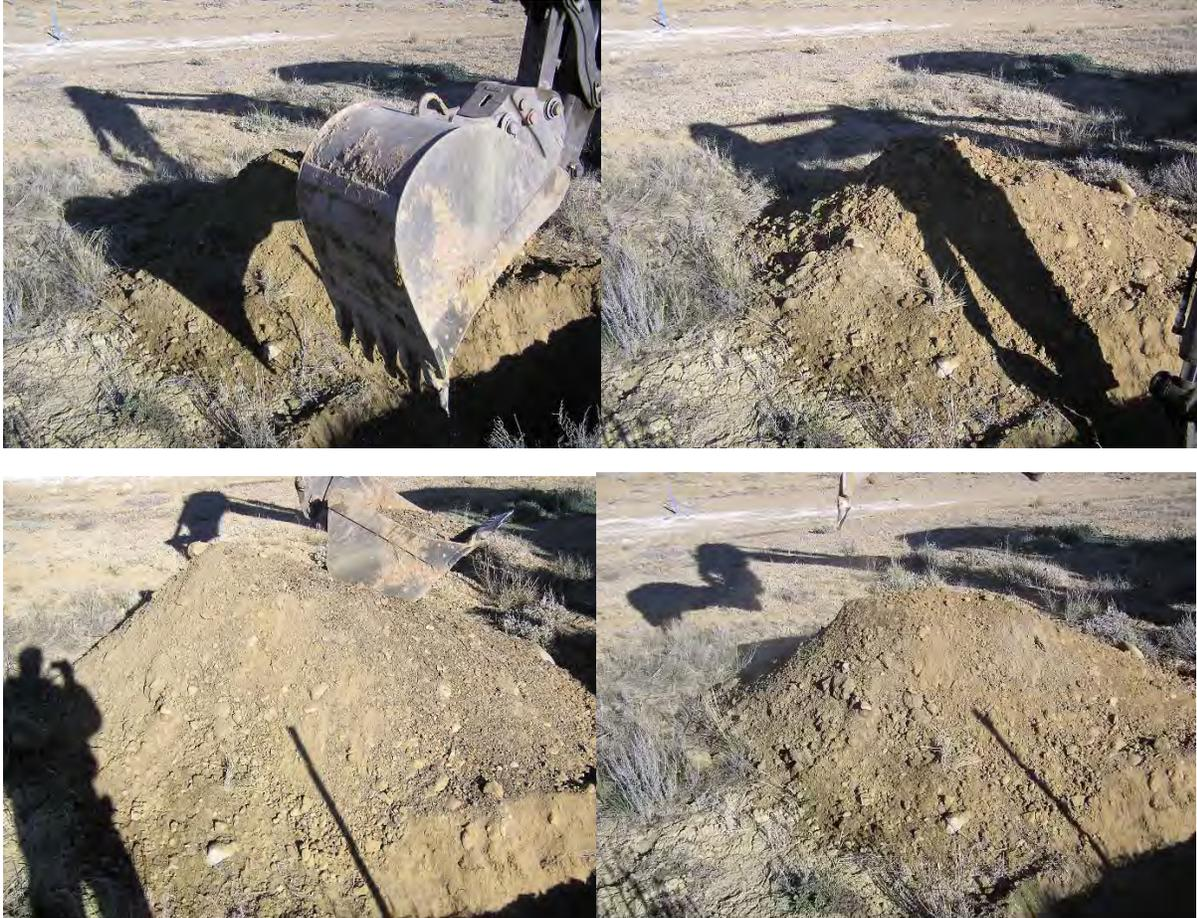
0 to 2 ½ Feet the material was generally consistent with that of a silty sand (SM) material. 2 ½ - 5 feet the material was a pit run cobble material (SM). 5 – 7 feet the material turned to a decomposed shale material.
