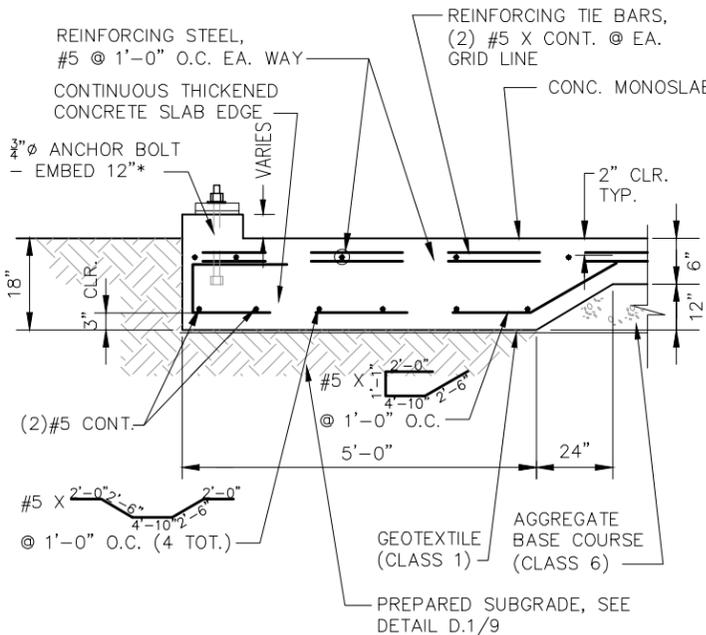
NOTE: REFER TO FOUNDATION PLAN FOR SLAB SLOPE AND CONTROL/CONSTRUCTION JOINT LOCATIONS.
