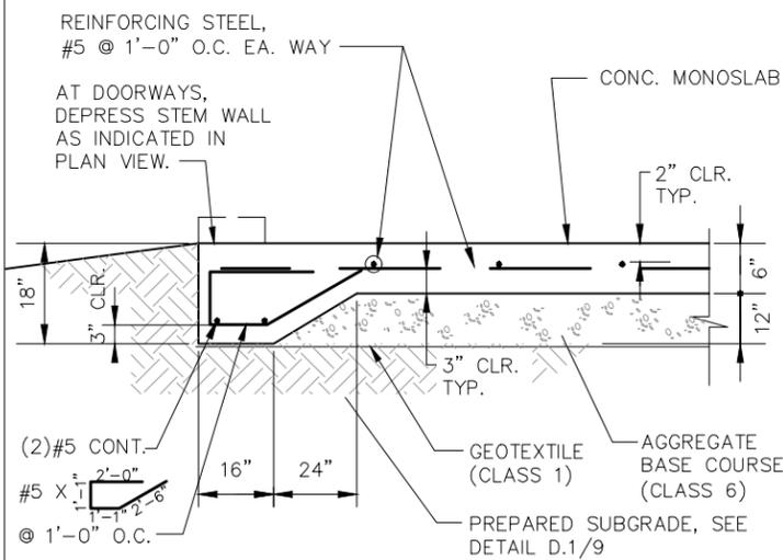
NOTE: REFER TO FOUNDATION PLAN FOR SLAB SLOPE AND CONTROL/CONSTRUCTION JOINT LOCATIONS.
