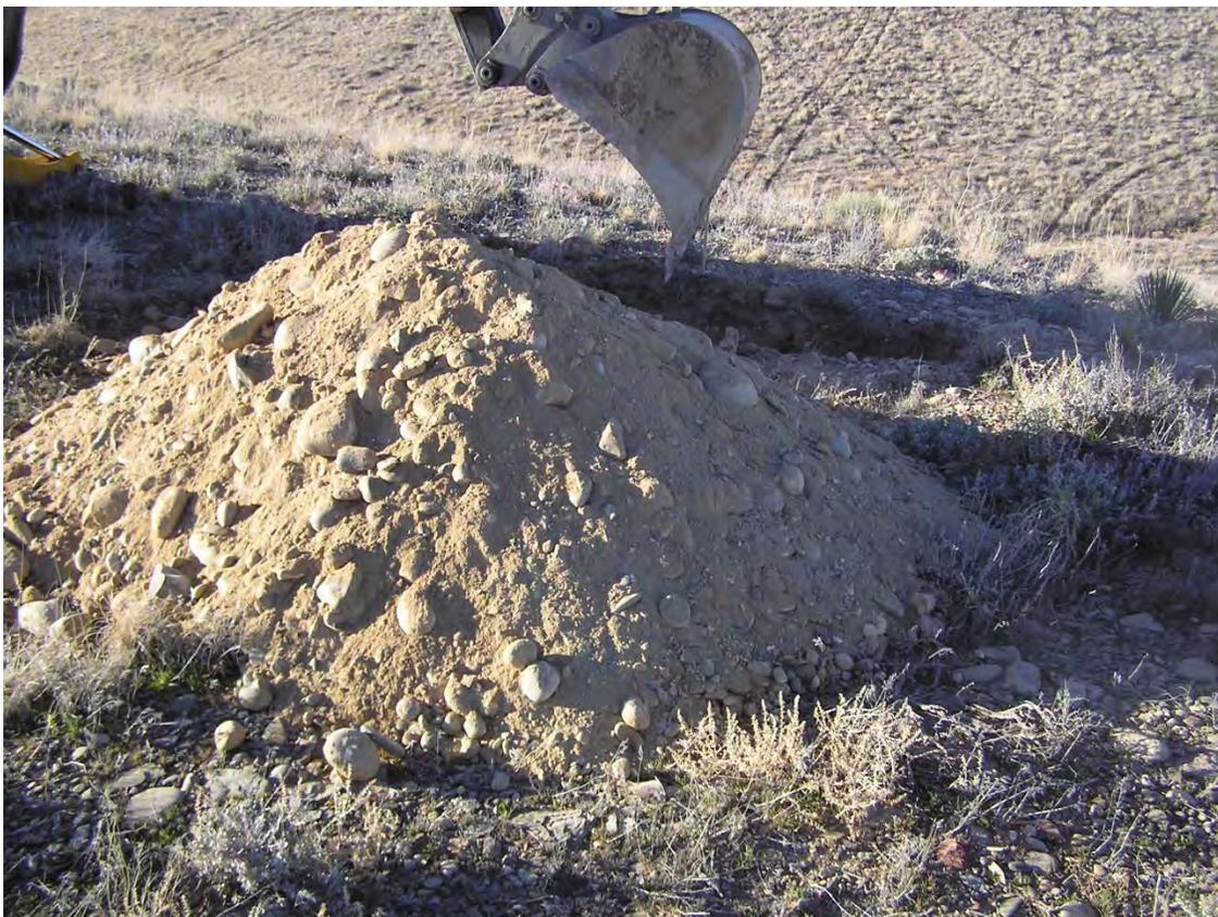
The full depth of the test hole to 5 feet consisted of pit run cobble material poorly graded with a sand-silt mixtures (SM).
