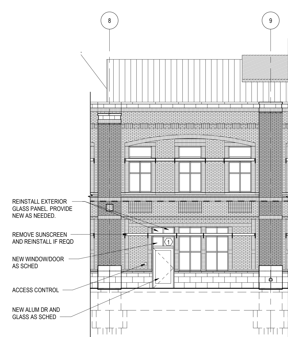
3 SOUTH ELEVATION - CONSTRUCTION A5-1 1/8" = 1'-0"
