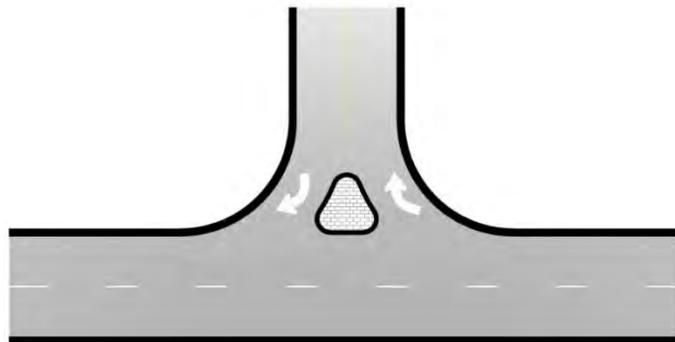
*Right-in/right-out with channelizing island eliminates left turn movements at specific locations.*
