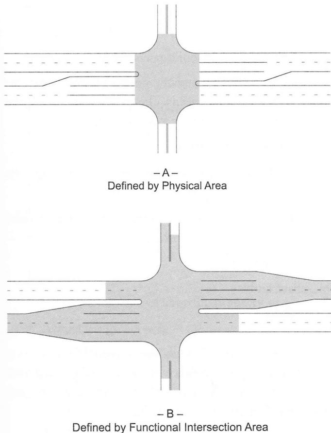
Figure 9-2. Physical and Functional Area of an Intersection
