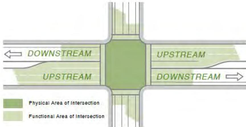
The functional intersection area will depend on the speed of the segment and the number of projected turning vehicles. As an example, in a 45-mph suburban section with a maximum of 100 turning vehicles during the peak hour, the upstream and downstream functional intersection areas (FIA) are as follows:
