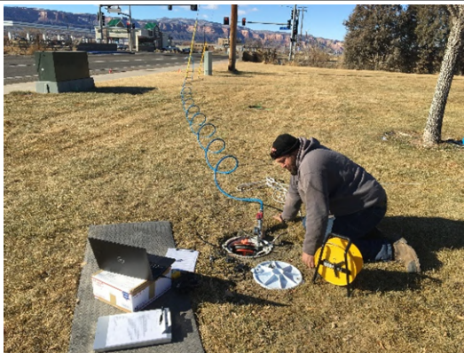
FIGURE: 5 – Drawdown test in TW-1.
