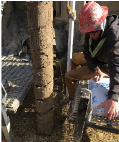
FIGURE: 3 – Clay soil stuck to augers (BH#2).
