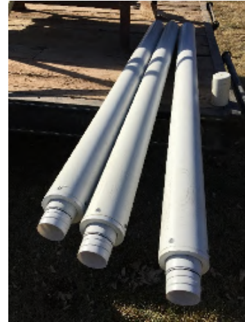
FIGURE: 2 – Sample prepacked well pipe.
