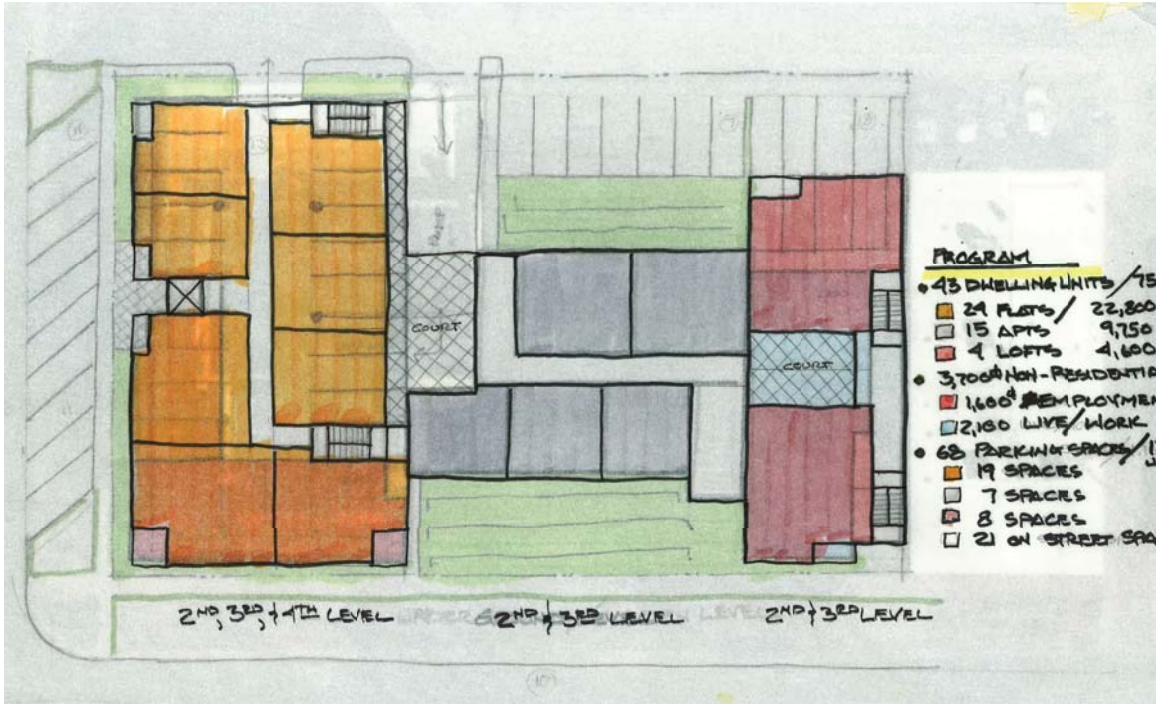
Image 9. Floor plan showing the proposed layout of the second/third levels of White Hall.
