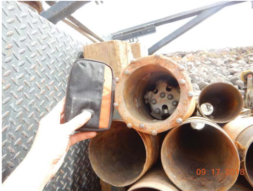
Figure 7. Symmetrix drive casing advancer bit. Camera case is 6-inches long for scale.
