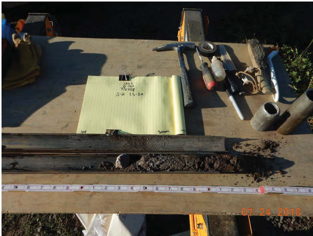
Photograph 16: B-102A(P); S-2 from 1.5 to 3.0 feet. Clayey Gravel with Sand [Fill].
