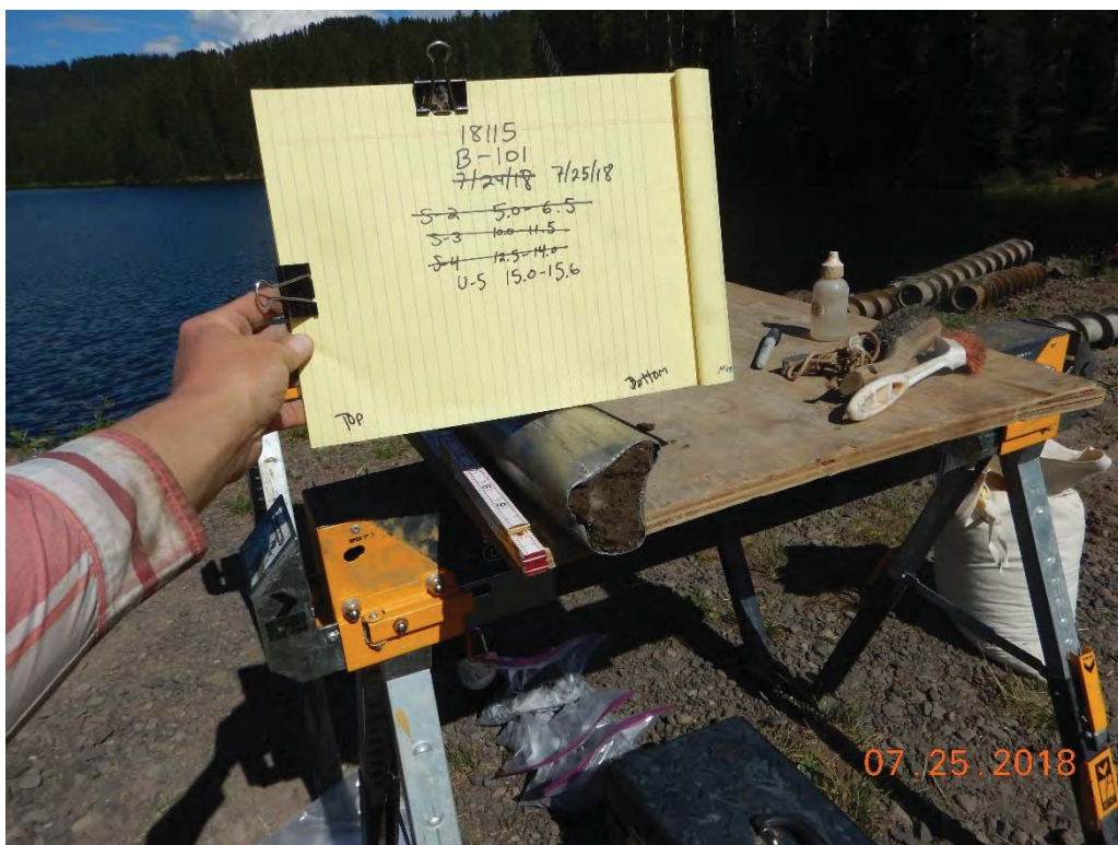
Photograph 4: B-101(P); U-5 from 15.0 to 15.6 feet. Disturbed. Clayey Sand with Gravel [Fill].
