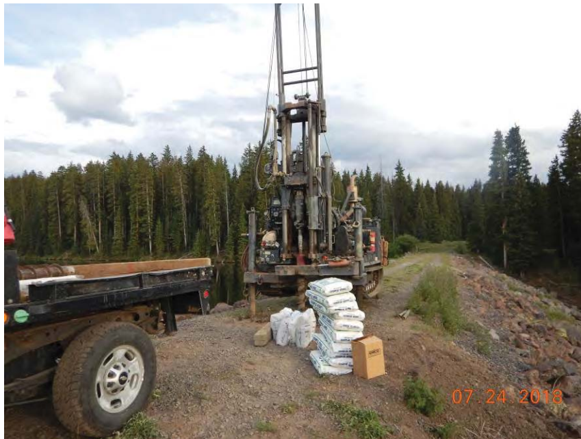
Figure 3. B-102A at the end of day, looking southeast. Auger casing rod is attached to in-place augers.
