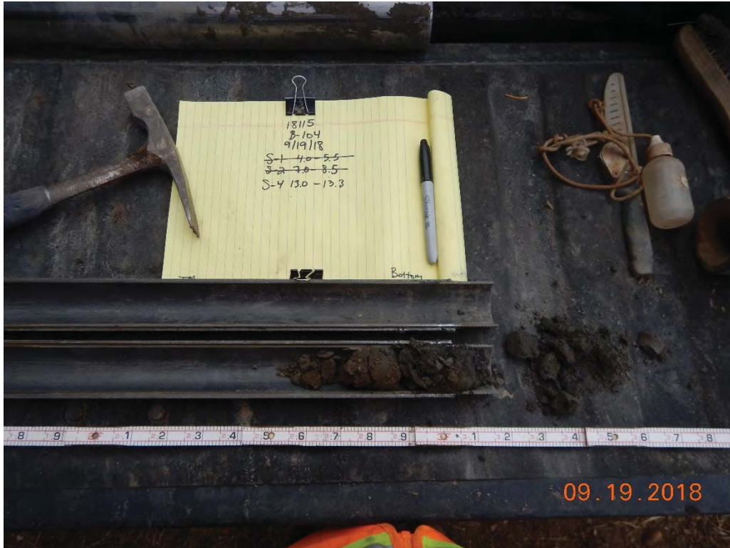
Photograph 43: B-104(P); S-4 from 13.0 to 13.3 feet. Gravelly Lean Clay with Sand [Alluvium/Colluvium].
