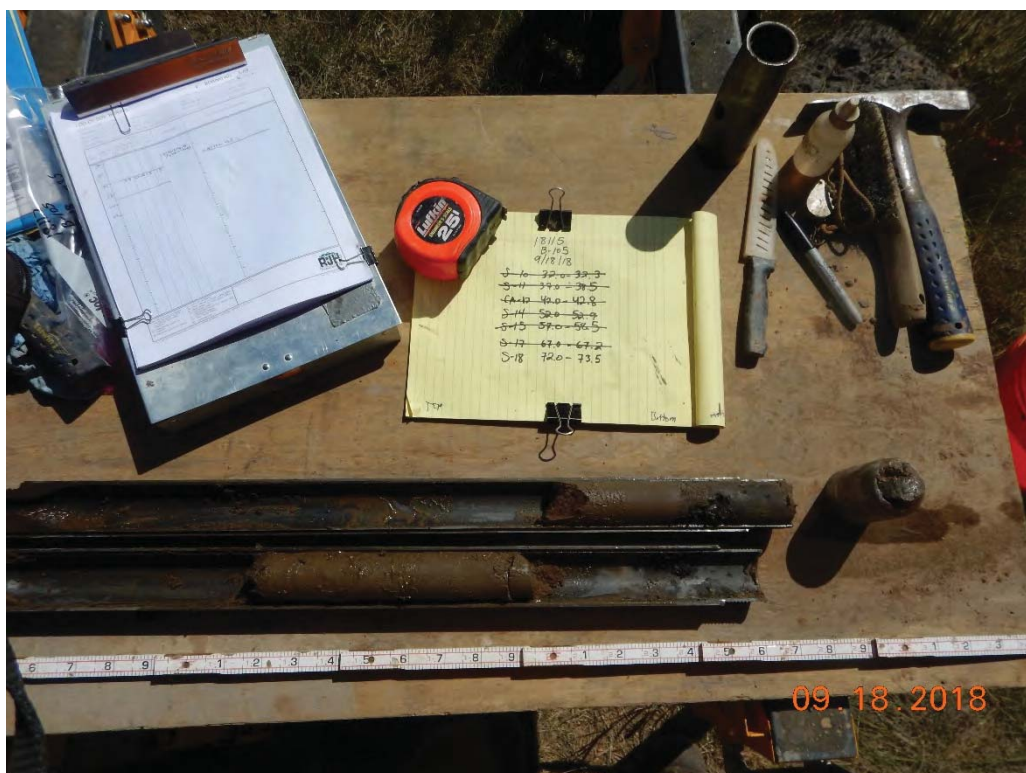
Photograph 61: B-105A(P); S-18 from 72.0 to 73.5 feet. Clayey Sand with Gravel [Alluvium/Colluvium].
