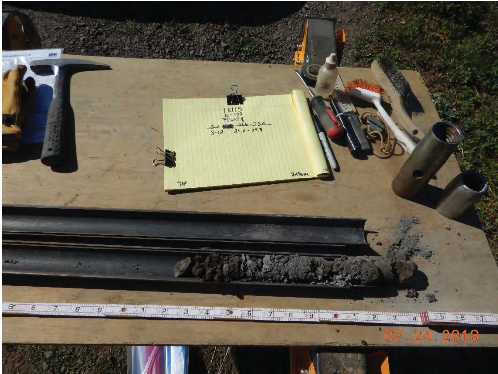
Photograph 24: B-102A(P); S-12 from 24.0 to 24.8 feet. Clayey Gravel with Sand [Fill].
