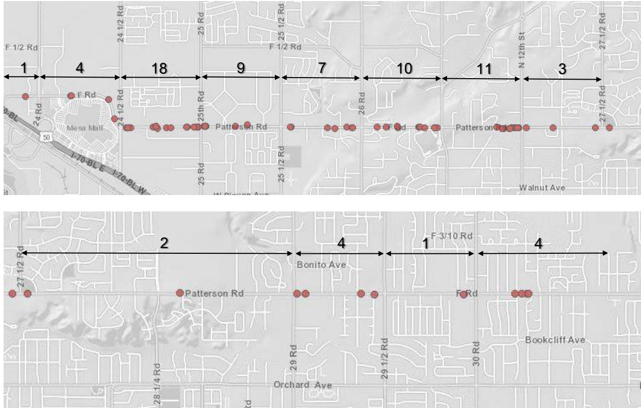
Figure 2. Patterson Rd Driveway Crashes
