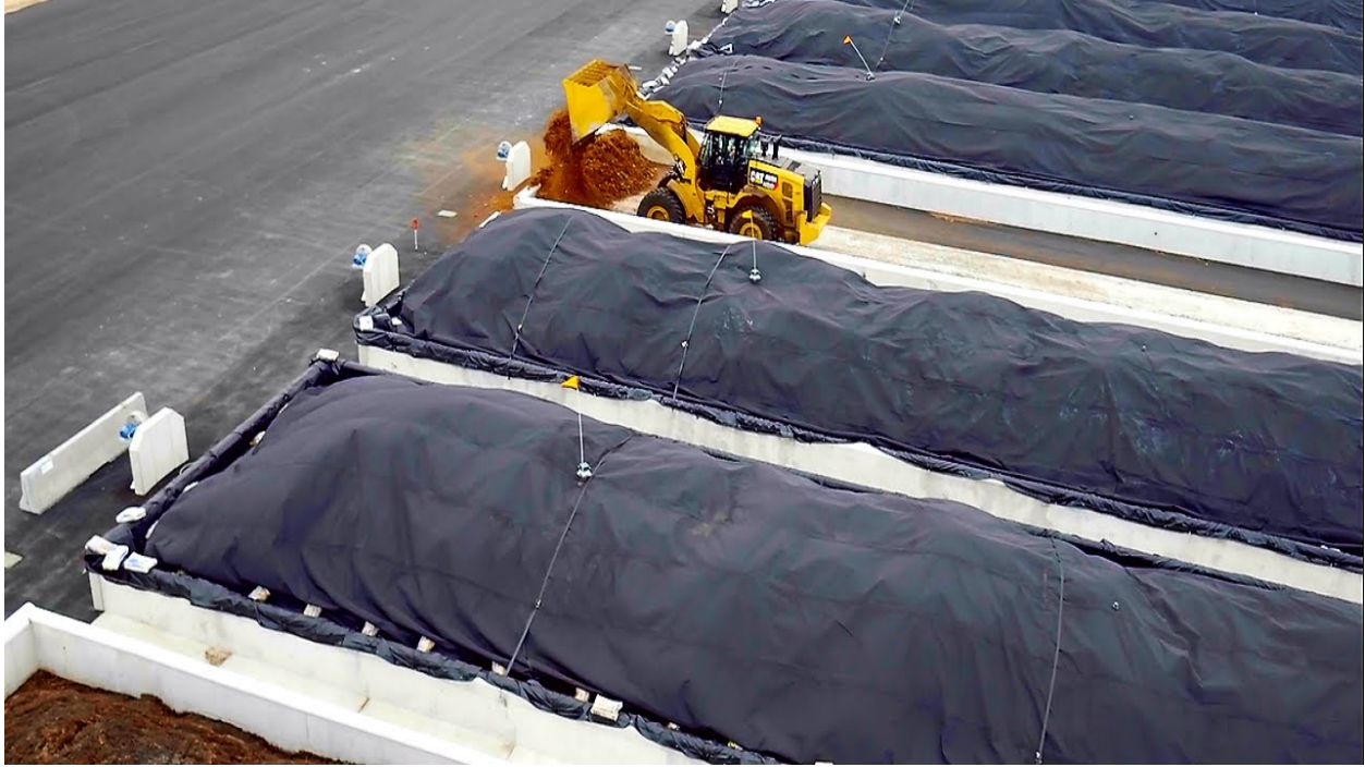
Figure 6.4 Aerated Static Pile Composting
