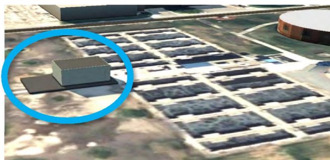
Figure C-3. Our recommendation is to put the new blower building on top of an extension of the RAS/WAS pumping gallery, which would be extended southward.
