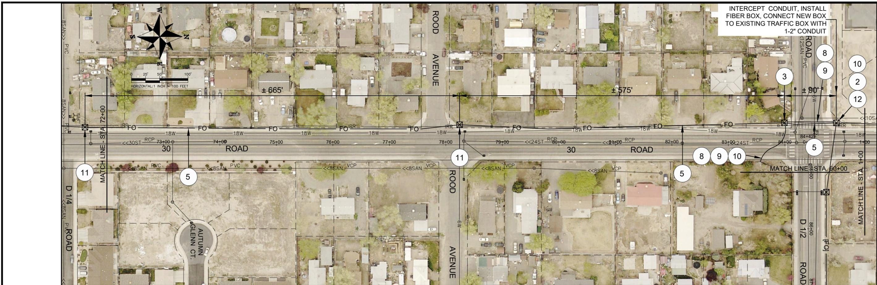
INTERCEPT CONDUIT, INSTALL FIBER BOX, CONNECT NEW BOX TO EXISTING TRAFFIC BOX WITH 1-2" CONDUIT
