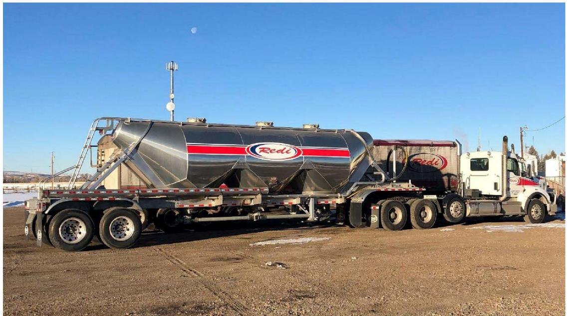
*Figure 2 Pneumatic Transport, Rock Dust, Sodium Bicarbonate*
