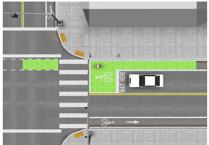
FIGURE 29: BIKE BOX AT INTERSECTION
