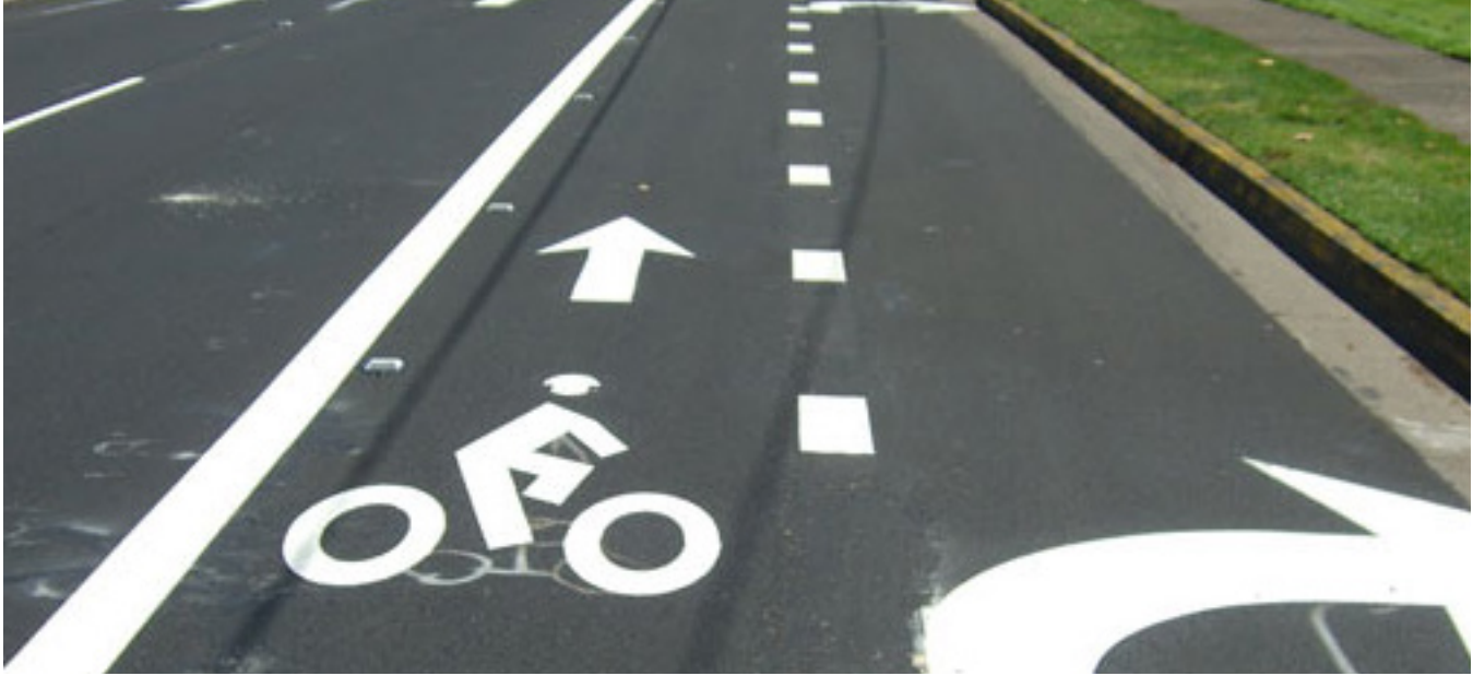
FIGURE 26: COMBINED BIKE LANE/TURN LANE
