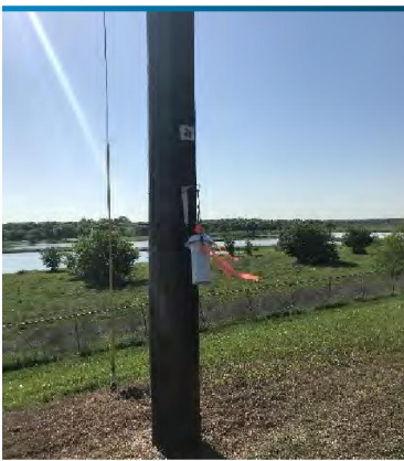
Fenceline (ppbv) H2S monitors can be deployed to assess potentially detectable odor levels at the plant fenceline and in surrounding neighborhoods.
