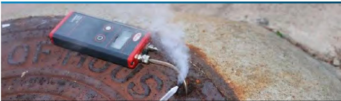
Surface-level smoke tests and differential pressure measurements can help identify pressurized headspaces in collection systems. Pressurization can sometimes be measured well over a mile upstream of a headspace constriction point.
