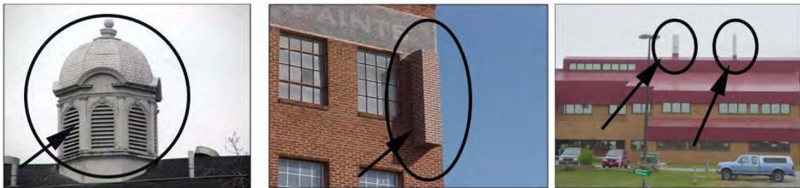
Figure 6: Examples of Antenna Concealment Techniques
