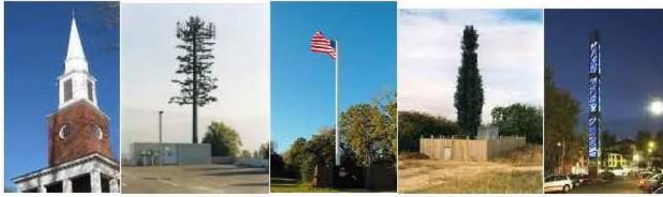
Figure 04.03-3 Examples of Concealed Facilities
