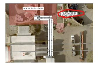
**A:** The penetration will be "constructed by others" prior to the installation of the belt. Essentially, the building will be fabricated with a 4'x4' opening.
