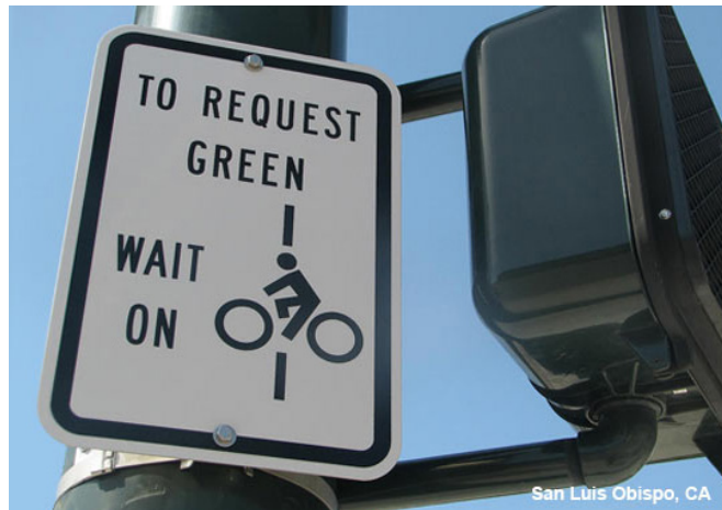
FIGURE 27: BIKE DETECTION AT SIGNAL
