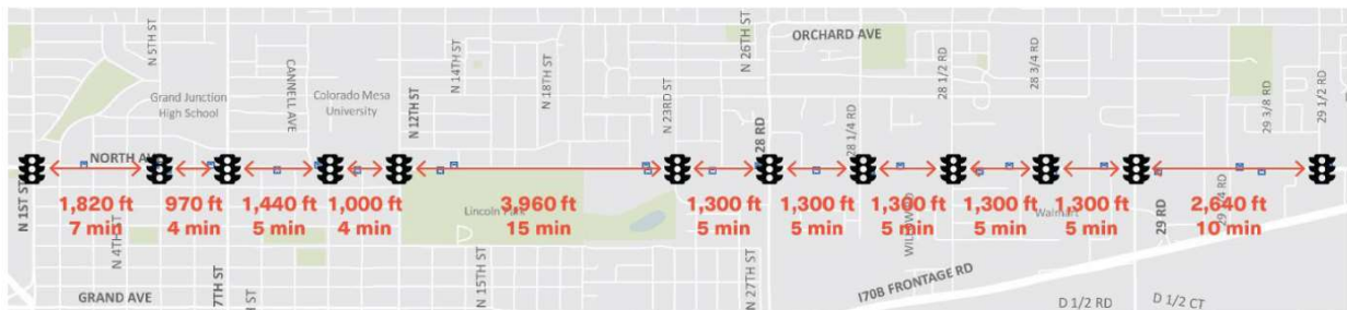
Figure 8 - Signal Spacing on North Avenue (Source: North Avenue ETC Study, Technical Team Meeting #3, December 6, 2021)
