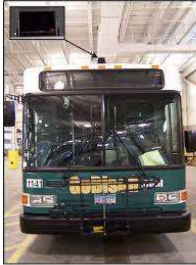
Figure 7 - Bus Equipped with GTT Opticom LED Emitter (Source: Advanced Traffic Analysis Center)
