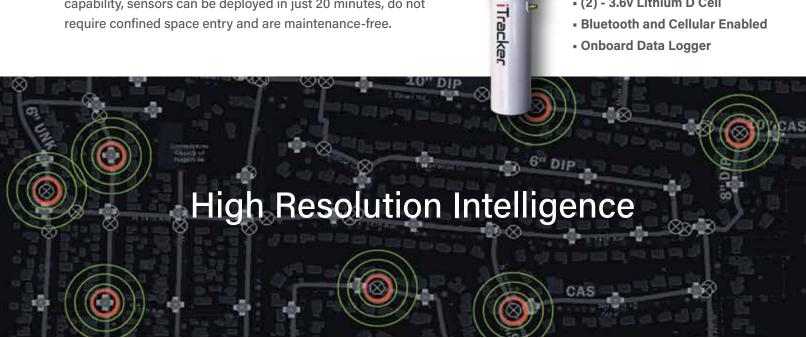
iTracker Smart Sensors deliver a network of high resolution data points that quickly pinpoint I&I down to a set of adjoining manholes.
