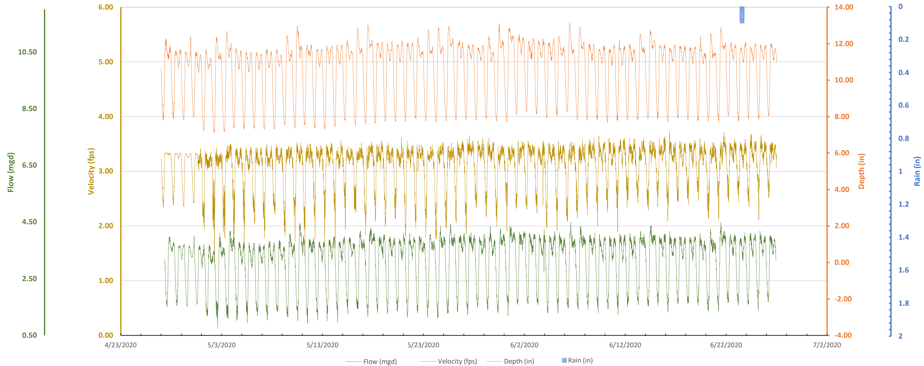
GJ02 D, V, Q & Rain Hydrograph (Pipe Inside Diameter=28.88")
