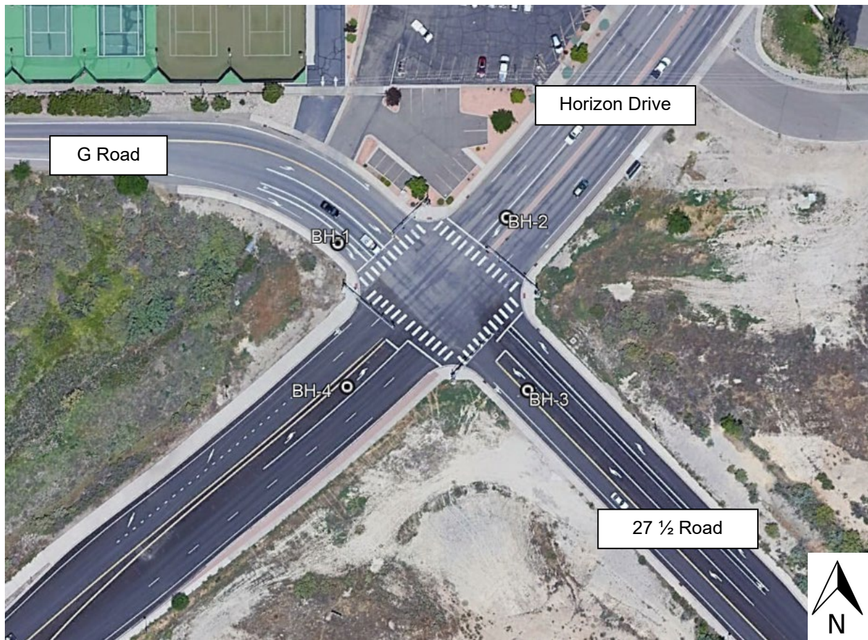
Figure 3 – Borehole Location Plan (Google Earth)
