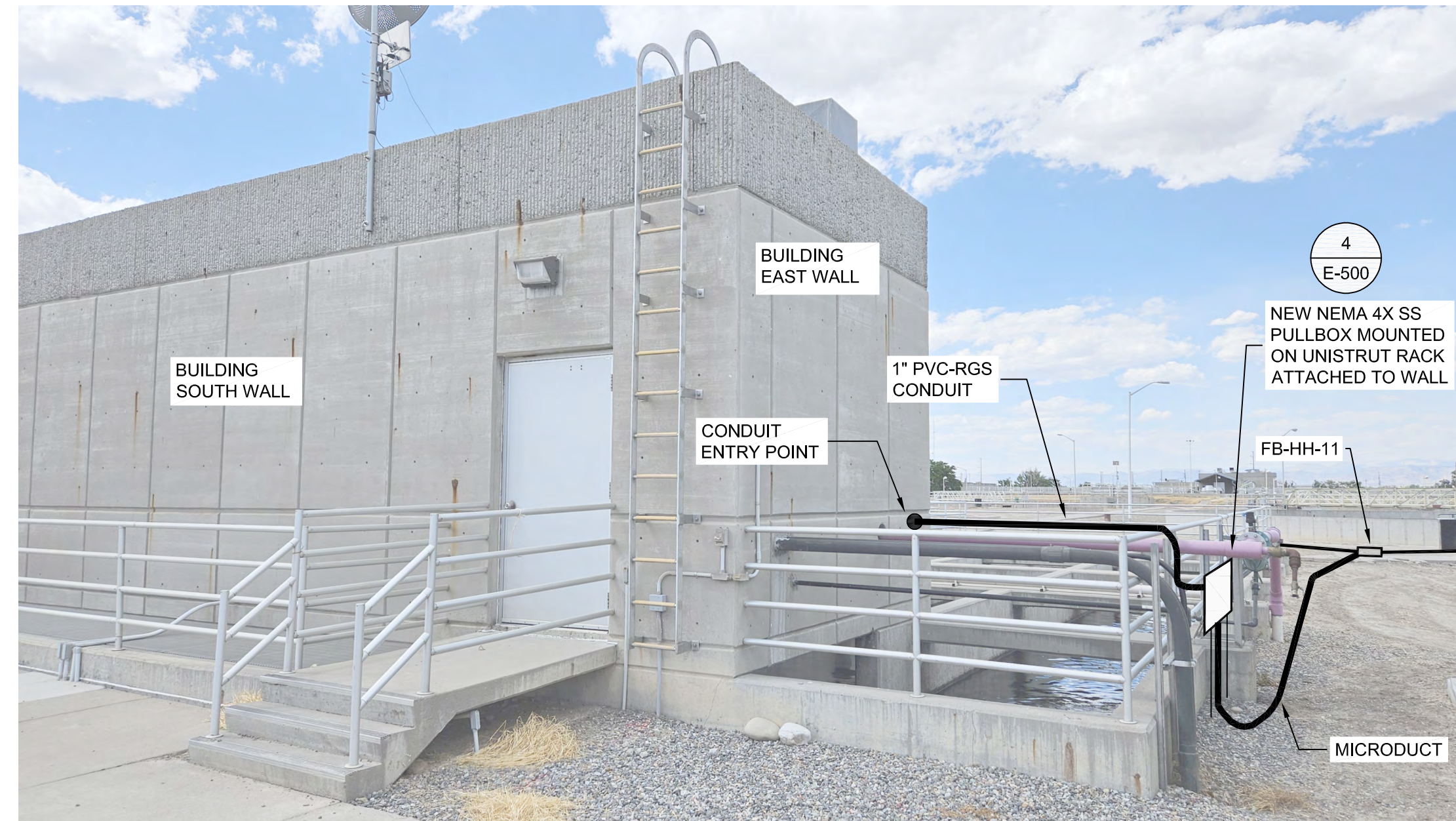
1 PLANT WATER BUILDING EXTERIOR MICRODUCT/CONDUIT ROUTING
