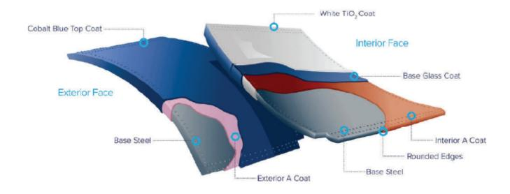
Vitrium™ is the world's leading glass-fused-to-steel coating for bolted storage tanks and has been proven in the field for more than 67 years. CST's Vitrium coating technology enhanced with titanium dioxide (TiO₂) is applied in a 3-coat, 1-fire (3c1f) process procedure. Vitrium is also produced in a 3-coat, 2-fire (3c2f) process primarily when special colors are requested or thicker layers of glass are required.
