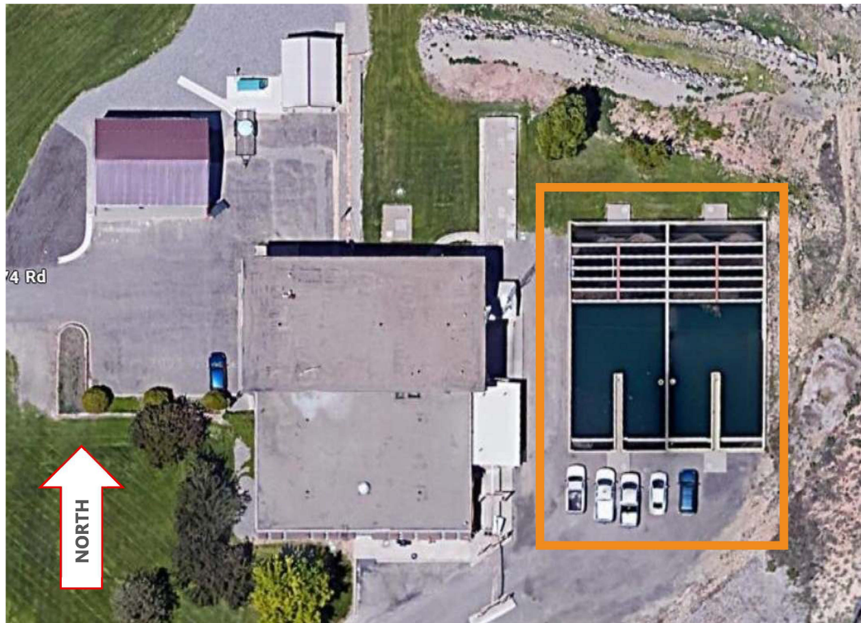
Figure 1. Contact basins (orange highlight) at the City's drinking water treatment facility. Note baffles at north end.
