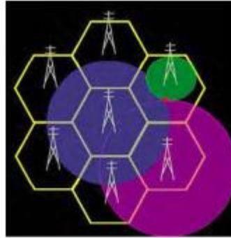
Hexagonal Grid with Circular Coverage from a Tower or Base Station (Image: 5freshminutes.IT)
