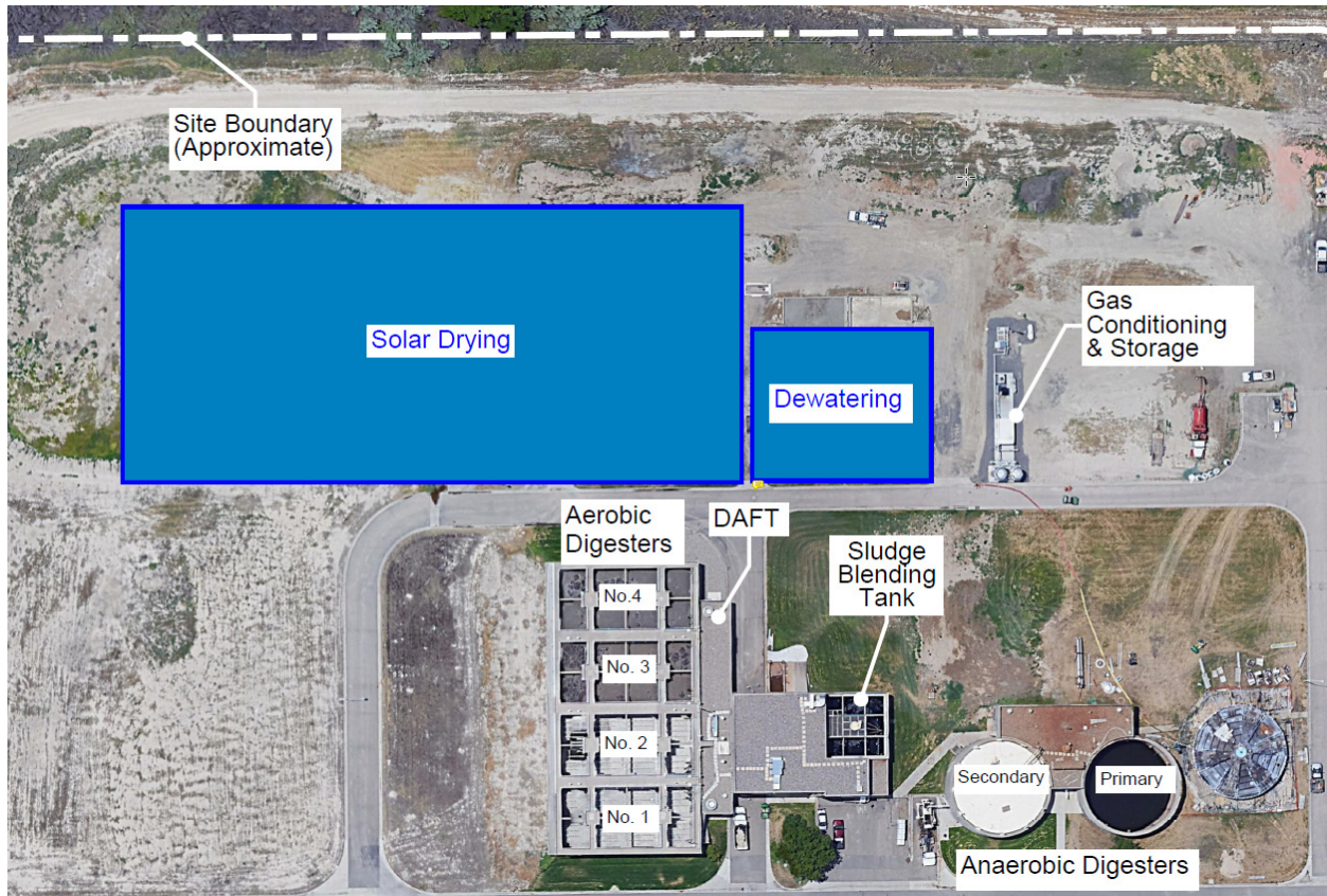
Figure 5.39 Proposed Screw Press + Solar Drying Layout
