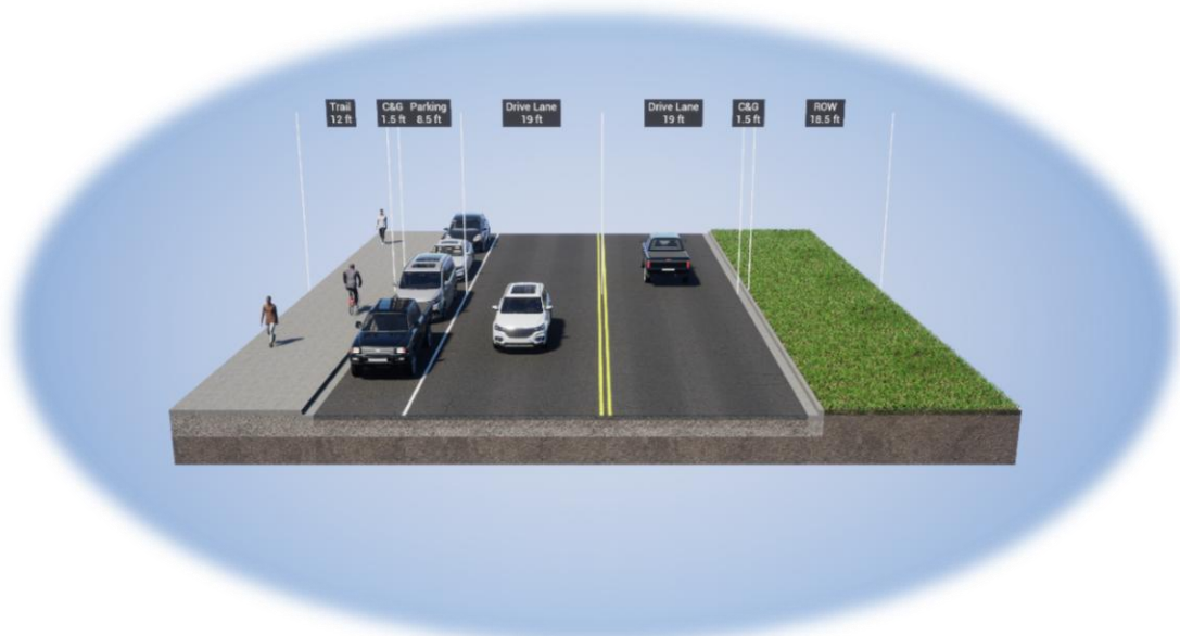
Figure 3 – 9 th Street Western Shared Use Trail Cross Section from Riverside Pkwy to Ute Ave Parking Constrained (80ft ROW)
