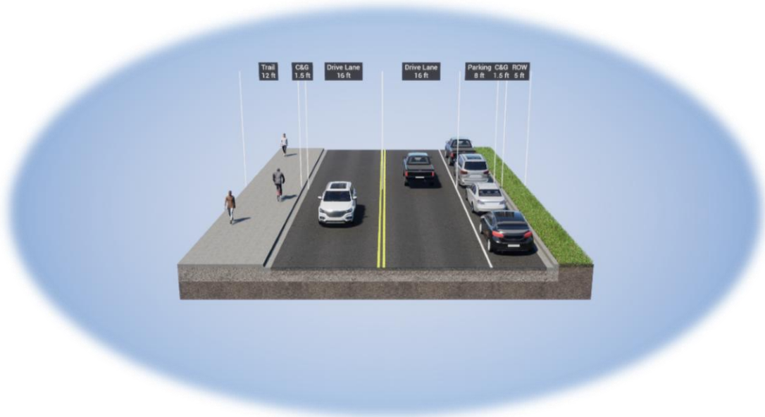
Figure 4 – 9 th Street Western Shared Use Trail Cross Section from Riverside Pkwy to Ute Ave ROW Constrained (60ft ROW)
