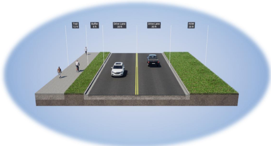
Figure 3 – 9 th Street Western Shared Use Trail Cross Section from Riverside Pkwy to Ute Ave Parking Constrained (80ft ROW)
