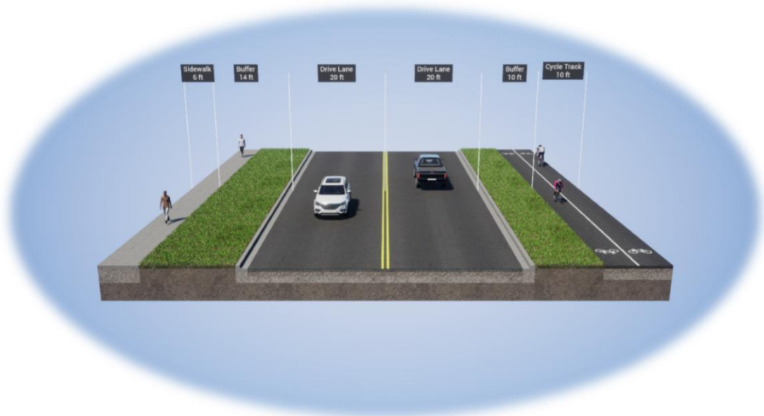
Figure 5 – 9 th Street Eastern Cycle Track Cross Section from Riverside Pkwy to Ute Ave
