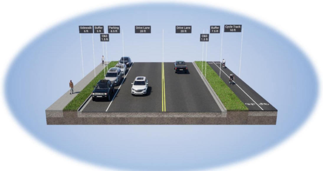
Figure 7 – 9 th Street Eastern Cycle Track Cross Section from Riverside Pkwy to Ute Ave ROW Constrained (60ft ROW)
