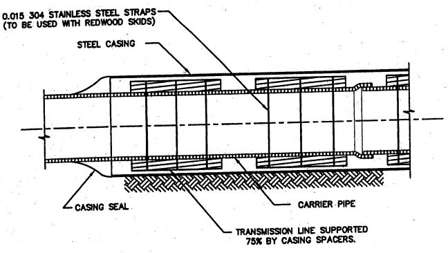
NOTE: CASING SPACERS MAY BE EITHER REDWOOD OR STAINLESS STEEL PIPE INSULATORS WITH POLYMER RUNNERS.
