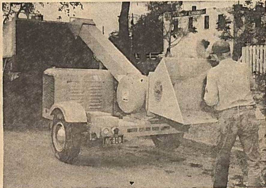
The Forestry division uses a chipper in maintaining trees in residential parkings and in the parks. Each year all trees are trimmed and sprayed as required to keep them healthy. Use of the chipper results in more efficient handling of branches and twigs.
