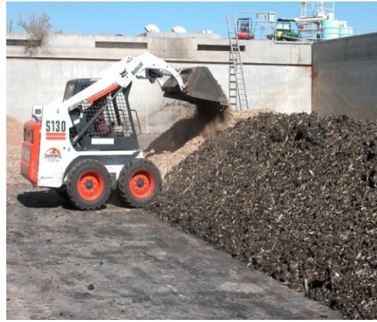
Covering pile with woodchips
