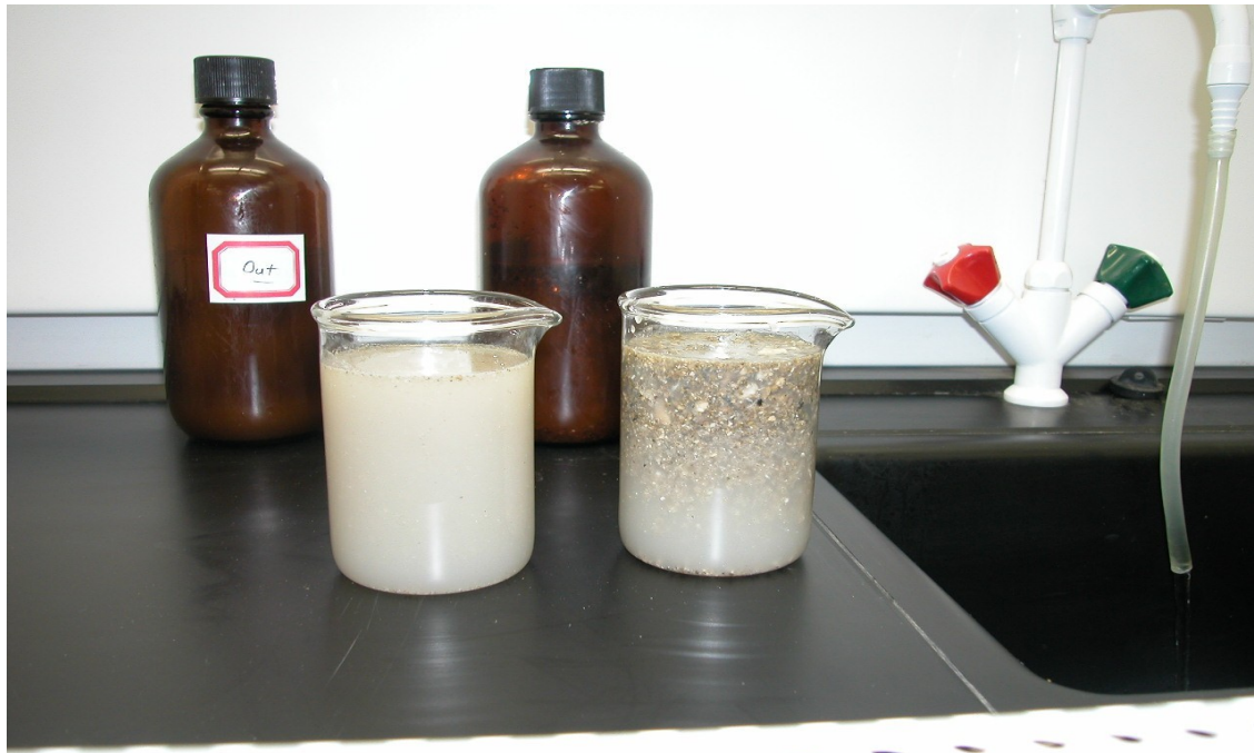
Liquid Samples: Influent to grease removal unit (right). Effluent from unit (left)
