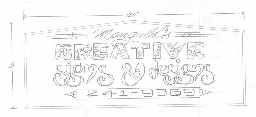
CONSTRUCTION: 1/2" X4 X10" M.D.O. BOHRD (39 50 FT.)
