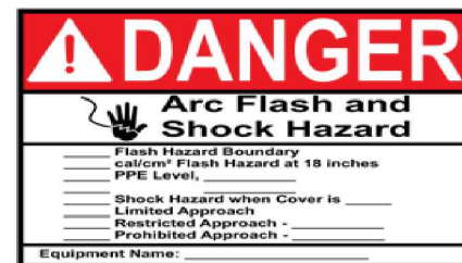
Typical sign required by NFPA 70E by ComplianceSigns.com
