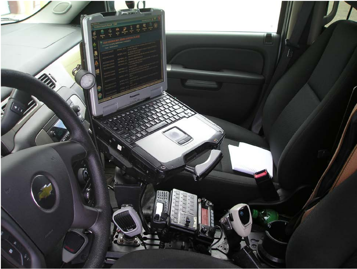
Chevy Tahoe – Havis dock, 9" Gamber-Johnson pole and quad-motion attachment
