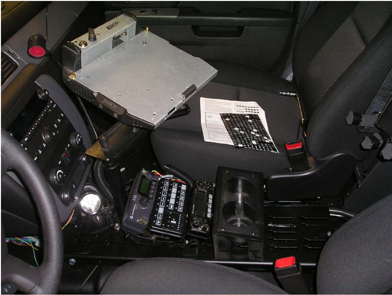
Chevy Tahoe – Havis (Ledco) dock with attachment, 9" Gamber Johnson pole
