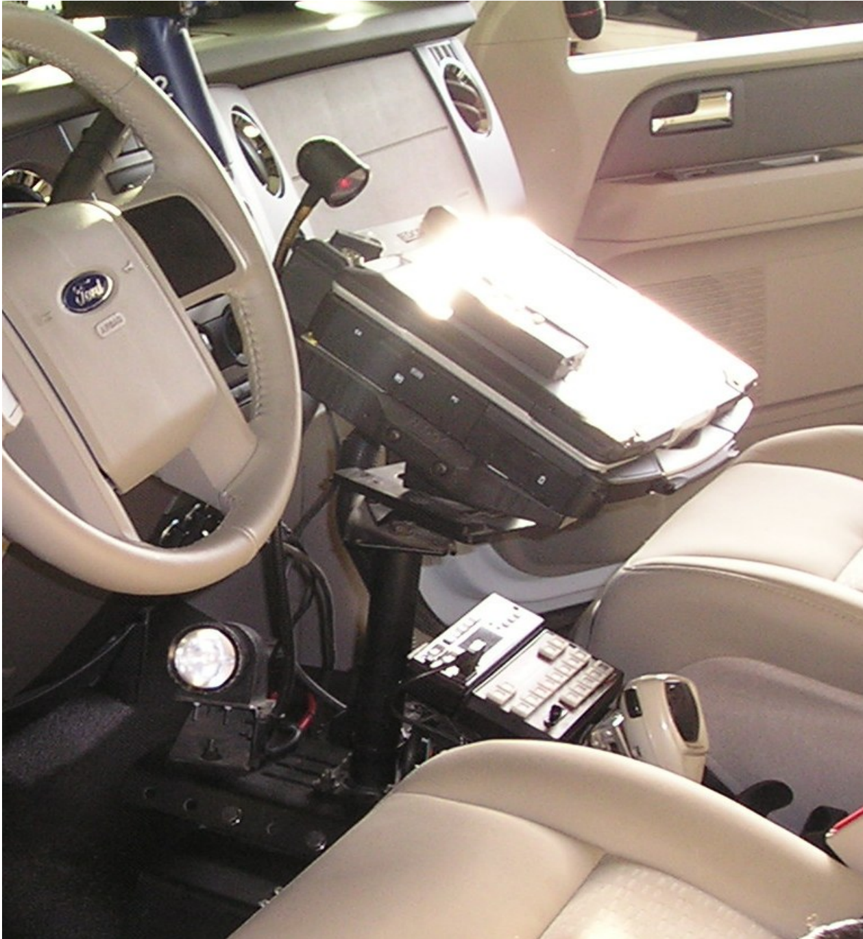
Ford Expedition – Havis dock, 9" Gamber Johnson pole with quad-motion attachment below the dock
