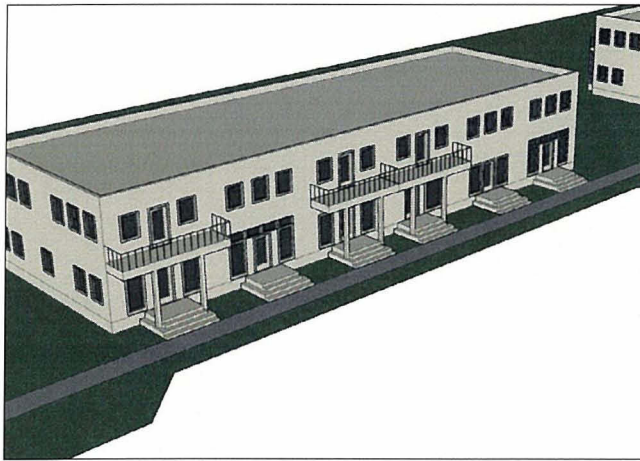
Conceptual massing model: Live/Work, Perspective A depicts strong relationship between from building facade and sidewalk as a result of a "0" setback.
