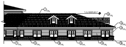
MEMORY CARE ADDITION NORTH ELEVATION SCALE: 1/8" = 1'-0"
