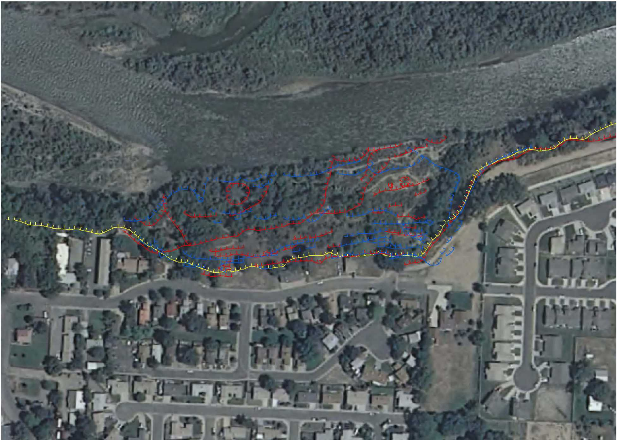
Figure 2. The Lamplite Landslide and surrounding neighborhood in a 2009 NAIP image. The yellow hachured line is the location of the 1950 headscarp and blue hachured lines are from the 1985 CGS study. The red hachured lines are scarps, pressure ridges, slumps, and depressions mapped in March of 2012.
