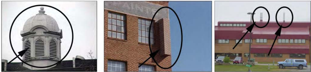
Figure 6: Examples of Antenna Concealment Techniques
