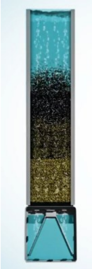
Example of air scour function during backwash
