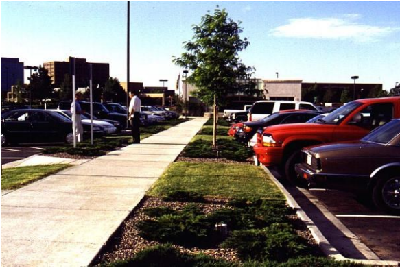
Sidewalks and landscaping break up and soften the visual impact of large parking lots
