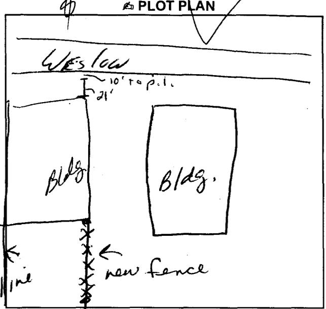
*36" high 21' long guardrail 2 7/8 galvanized pipe in front, 10' behind prop. line. Amended 4-11-97 SLK*
