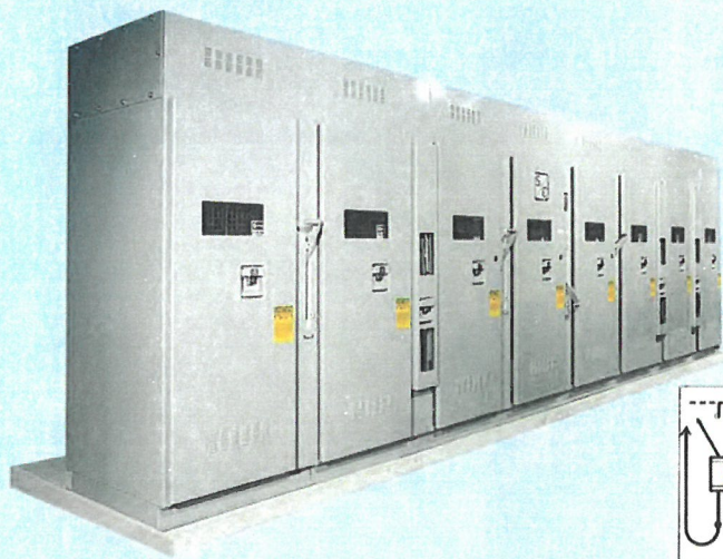
Figure 10. The manual, primary-selective, eight-bay lineup of S&C Custom Metal-Enclosed Switchgear pictured above is configured in a split-bus arrangement. Each bus section is supplied power through a normally closed incoming switch, with the bus-tie switch normally open between the bus sections. Three-phase load circuits are switched and protected by power-operated S&C Interrupter Switches with Power Fuses. Automatic trip-open operation of these switches is initiated by S&C Open-Phase Detectors on single-phasing resulting from blown feeder fuses or from source-side open-phase conditions at the same system voltage as the metal-enclosed switchgear. Three-phase voltage sensing for each power-operated switch is provided by S&C Voltage Sensors. Manually operated S&C Interrupter Switches with Power Fuses switch and protect single-phase load circuits. Provisions for future bus extensions are included.
