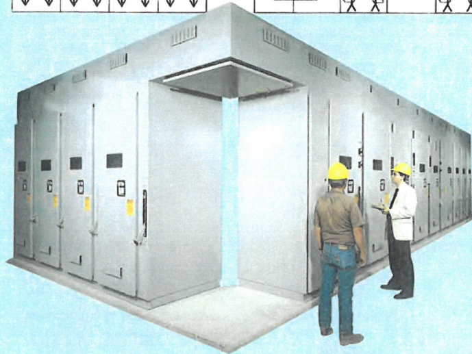
Figure 9. Fifteen bays of S&C Custom Metal-Enclosed Switchgear (pictured at left and diagrammed above) are arranged in an "L" configuration and serve as a power-operated split-bus primary-selective service-entrance switching center. Automatic switching of the two source switches and the bus-tie switch, by means of S&C Switch Operators and an S&C Source-Transfer Control, assures service continuity for the feeder circuits. Normally, the bus-tie switch is open and the bus sections receive power from independent sources. Should one source circuit fail, the associated switch is automatically opened and the bus-tie switch is automatically closed, with the remaining source then serving all loads. Current sensors and voltage transformers provide sensing and control power for the source-transfer control and switch operators. The switchgear assembly also includes S&C Fault Fiter Electronic Power Fuses for bus protection and coordination with the feeder fuses, and other features providing enhanced flexibility and operating convenience.
