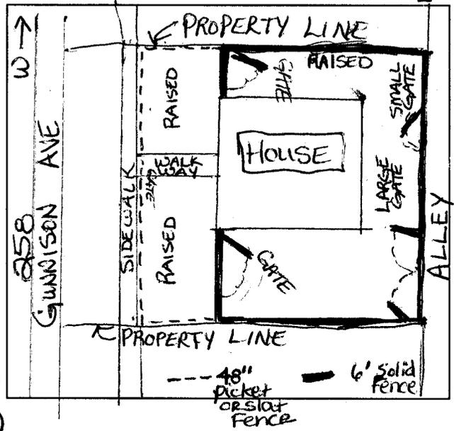
Plot plan must show property lines and property dimensions, all easements, all rights-of-way, all structures, all setbacks from property lines, & fence height(s). NOTE: PROPERTY LINE IS LIKELY ONE FOOT OR MORE BEHIND THE SIDEWALK.
