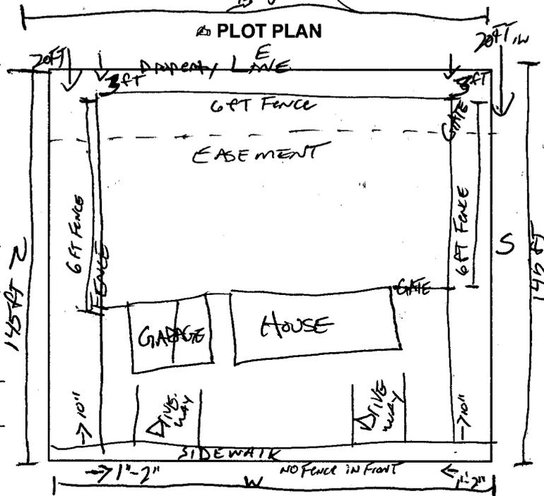
Plot plan must show property lines and property dimensions, all easements, all rights-of-way, all structures, all setbacks from property lines, & fence height(s). NOTE: PROPERTY LINE IS LIKELY ONE FOOT OR MORE BEHIND THE SIDEWALK.
