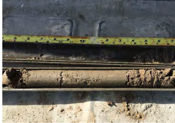
Photo 1 (left) shows the weathered shale found below 6.5 feet in BH#1 along Horizon Driver and Photo 2 (right) is the clay soil from a depth of 3 to 4 feet in BH#4 in the industrial portion of the project.
