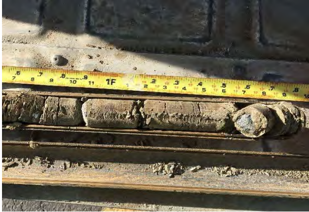
Photo 1 (left) shows the weathered shale found below 6.5 feet in BH#1 along Horizon Driver and Photo 2 (right) is the clay soil from a depth of 3 to 4 feet in BH#4 in the industrial portion of the project.
