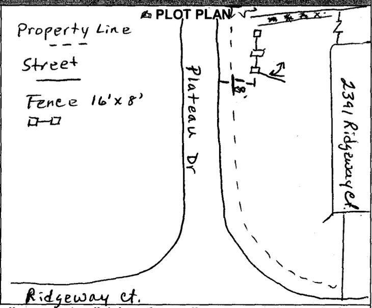
Plot plan must show property lines and property dimensions, all easements, all rights-of-way, all structures, all setbacks from property lines, & fence height(s). NOTE: PROPERTY LINE IS LIKELY ONE FOOT OR MORE BEHIND THE SIDEWALK.
