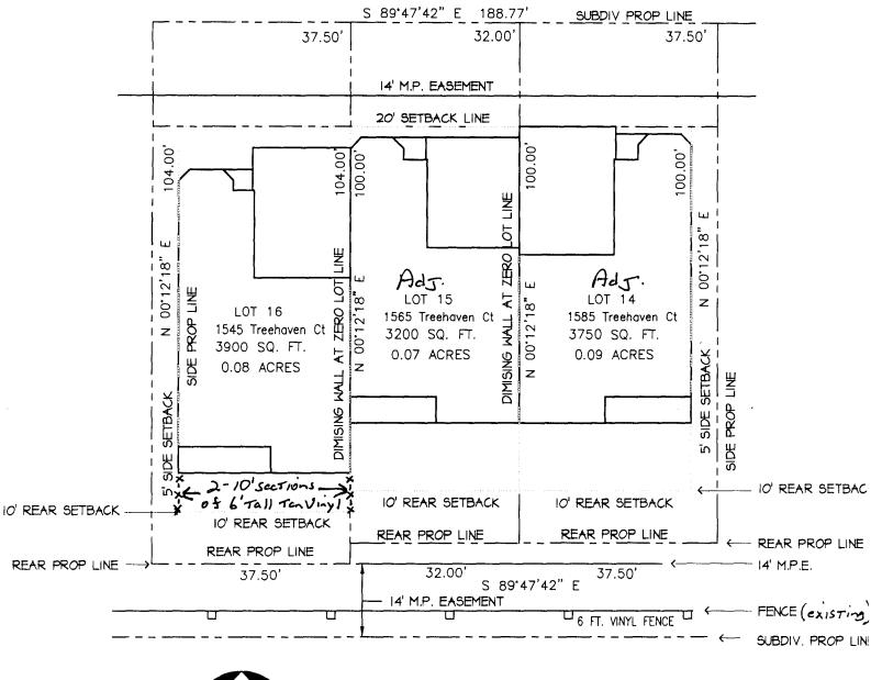
$\frac{\text{SITE PLAN}}{\text{NORTH}} \xrightarrow{\text{SITE PLAN}} JS 45$   $\frac{15 45}{\text{SCALE: I'' = 20'}} \text{Treehoven CT.}$   $\frac{1}{1000} = \frac{1}{1000} \text{Treehoven CT.}$   $\frac{1}{1000} = \frac{1}{1000} \text{Treehoven CT.}$
