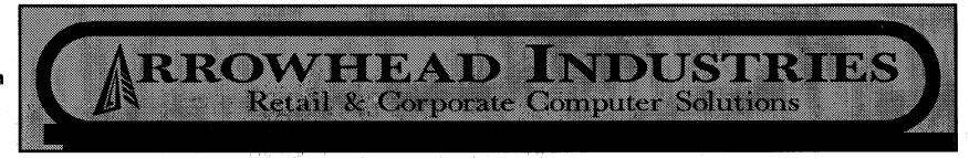
I in Industries 7.75 inches high R in Arrowhead is 6" High Border and Sign Frame are 3" in Width for a total of 6 Inches C in Computer is 4.125 inches
