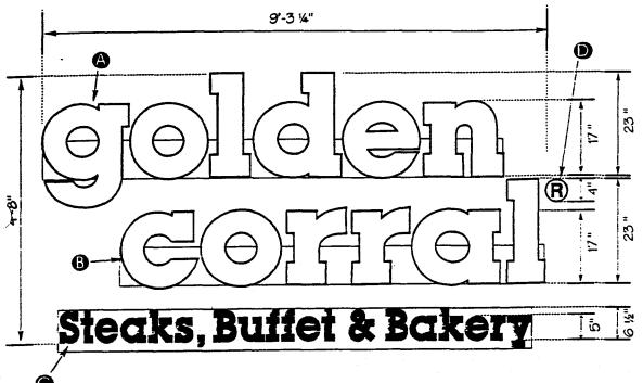
Sign contractor to wire to switched conductor provided in wireway (by electrical contractor) above ceiling. See electrical drawings to coordinate.
